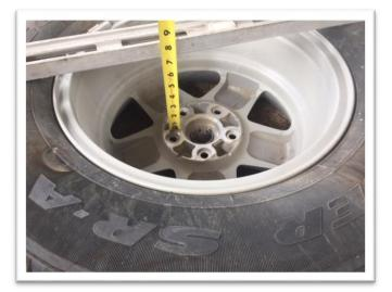
11. Subtract half an inch from the previous measurement, and set the tire carrier to the new measurement. This ensure tire is against the tire carrier.
