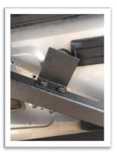
9. Install the rear tire carrier, securing it to the rear swing arm at the desire height using supplied hardware.
