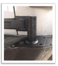
6. Install the carrier arm. First use a plastic bushing, then the carrier arm, then another plastic bushing, then the bracket to secure the carrier arm, and the c-clip.
