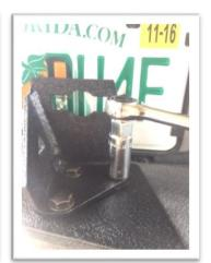
5. Attach the supplied bumper plate and carrier hinge to the passenger's side using the supplied Allen bolts. Ensure the side with the threaded bolt is facing up.
