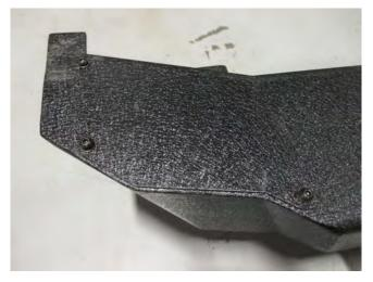
**STEP 5 //** Attach the supplied driver side bumper plate using the supplied allen bolts.
