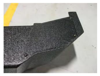
**STEP 6 //** Attach the supplied passenger side bumper plate using the supplied allen bolts.
