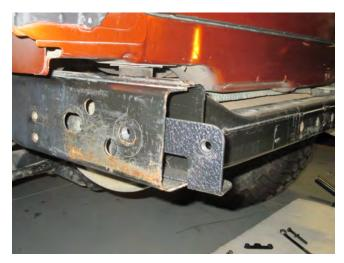
**STEP 2 //** Next, slide the L-Shaped mounting brackets into the frame rails with the nut backing up to the predrilled hole in the frame.
