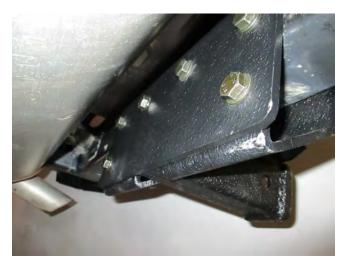
**STEP 4 //** Secure the backing plate, then tighten all bumper bolts that hold the bumper to the frame.
