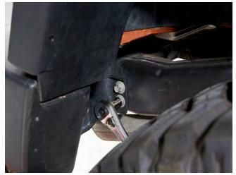
**STEP 1 //** Remove the (4) 15mm bolts securing the rear bumper.
