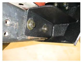
**STEP 3 //** Slide new rear bumper into place, securing the bump but leaving the bolts loose.
