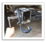
3. Place the L-Bracket into the end of the vehicle frame, with the threaded holes pointing away from the jeep so that the bumper will be held in place.
