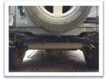
2. Remove 3 bolts that connect the OE tow hook, and then remove the OE tow hook.
