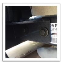
5. From behind the OE bumper frame, place the backing plate above the bumper and secure it.
