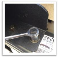
7. Attach the bumper plates using the supplied Allen bolts.
