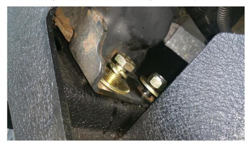
15. Using your ratchet and 19mm sockets (a deep socket is recommended here), tighten down all 6 lock nuts and both bolts. (the outer 4 bolts can be tightened from underneath the bumper and the inner 4 can be tightened down from the top) There is no recommended torque spec, so tighten them down completely.
