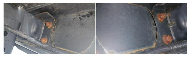
c. Using your 18mm socket (and extension, depending on how you want to position your ratchet), remove 6 bolts. These can be discarded, as they will not be used to install your new bumper, but for now, leave 1 bolt on each side attached loosely.
