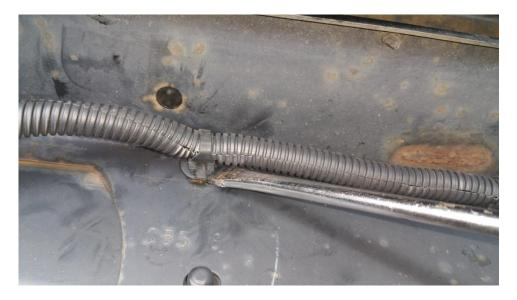
9. Once the wiring harness is disconnected, you can pull the stock bumper away. (wiring harness can be tucked up out of the way for now, either under the grille, or in the middle of the crash bar as shown below)
