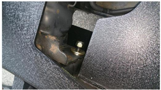
14. The remaining two empty holes in the plates are aligned with the grease packed holes (that have locknuts welded behind them). Take one of the 19mm bolts, thread on one split washer and then a flat washer, slide through the hole in the plate, and thread into the grease packed locknut that's integral to the bumper
