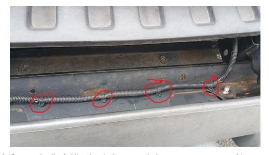
8. Use your utility knife to cut the clips holding the wire harness to the bumper, or use your screwdriver to pry them out.
