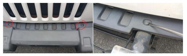
7. Go ahead and remove the last two bolts you left attaching the bumper to the frame and Very gently pull the bumper away from the frame rails to expose the wiring harness. DO NOT DROP THE BUMPER. You will have to support the bumper as you locate the 4 plastic clips securing the wiring harness to the bumper.
