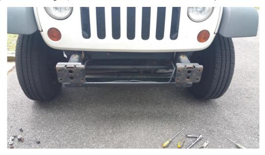
10. The existing crash bar needs to be trimmed, in order to be able to install the new bumper. Locate, and mark 1.5 inches from each of the ends of the existing crash bar.
