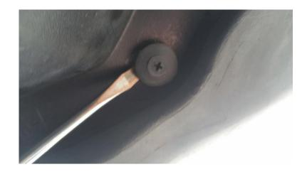
If you're not planning on reusing these fasteners, and prying with the screwdriver is difficult, feel free to yank them out with pliers, once you get them slightly pried out with the screwdriver
