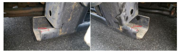
11. Using your hacksaw or cutoff wheel, remove the marked off 1.5" of material from the end of the crash bars (not pictured). Be sure to wear your protective gear as the cutoff wheel WILL create a shower of sparks, and potentially shards of metal. Below are pictures with the material removed.
