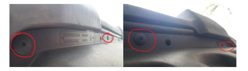
2. Using your flathead screwdriver, pry them out. If you're planning on reattaching the splash guard after the bumper installation, be gentle and save these for reuse (or purchase new ones at the auto parts store).
