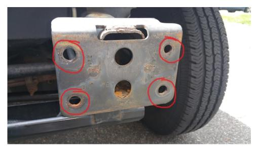
And on the inside of the bumper, find the corresponding bolts (and one empty bolt hole packed with grease – there's an integral lock nut welded behind the grease)
