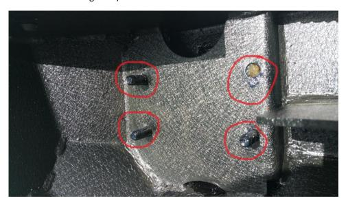
And slide the 6 integral bolts attached to the bumper through the corresponding bolt holes on the frame rails
