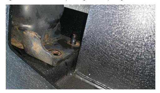
13. On each of the 6 integral bolts that are now through the plate on the end of the frame rails, slide on one of the flat washers, and one of the lock nuts
