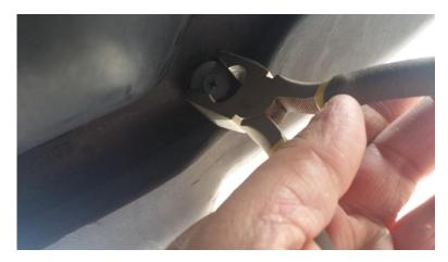
3. Once you get all four of those fasteners out, you'll see that there are two more attaching the splash guard to the crash bar. Remove these as well, and the splash guard will detach from the car.
