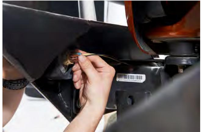
**STEP 8** // In most cases, the fog light harness will need to be extended. Cut and splice the wires to the appropriate length.
