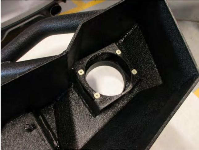
**STEP 5** // Insert the supplied plastic screw retainers.
