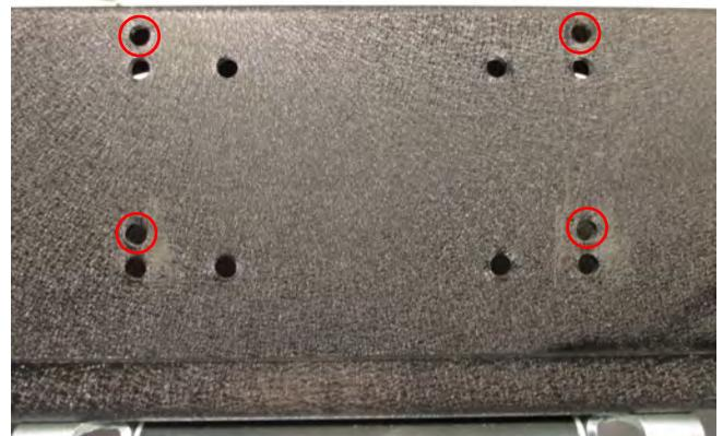
**STEP 10** // Line up the bolt holes with the rear most holes on the bumper. Using the bolts supplied with the winch, secure to winch to the bumper.
