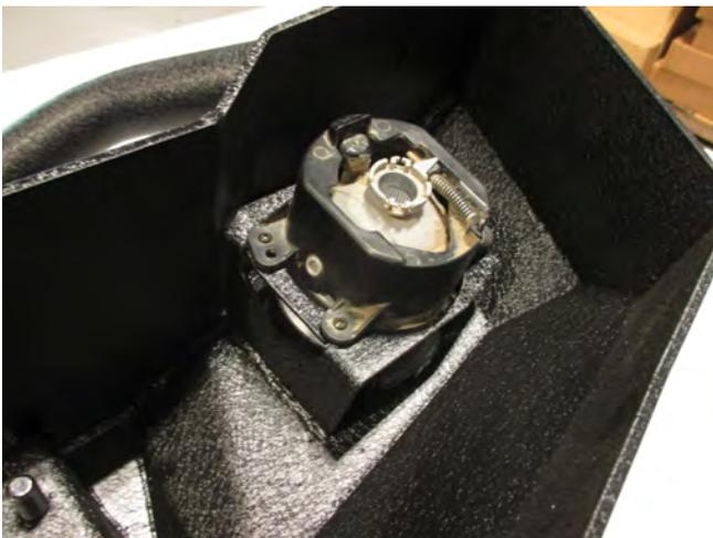
**STEP 6** // Using the supplied screws, secure the fog light housing to the bumper.
