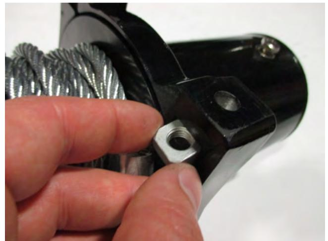
**STEP 9** // Insert the winch nuts into the winch housing.
