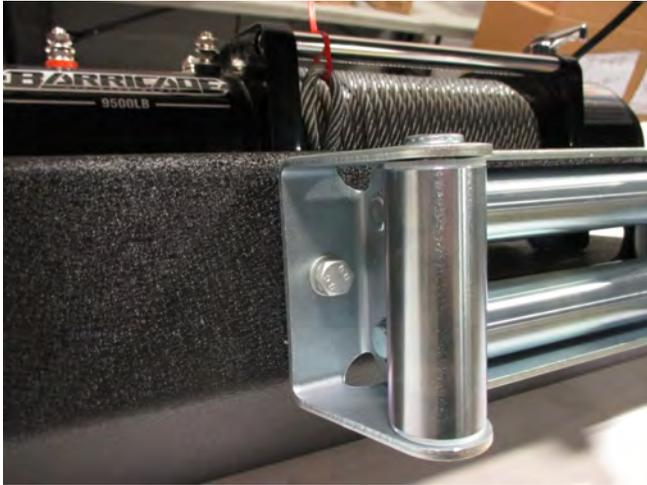
**STEP 11** // Attach the roller fairlead supplied with the winch using the 2 bolt holes on the front of the bumper.
