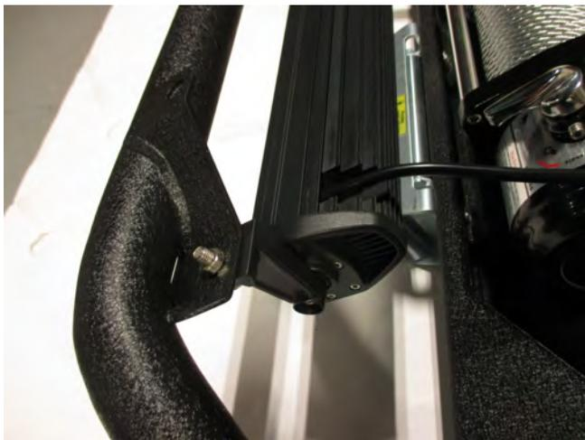
**STEP 12** // Install the LED Light bar using the brackets and hardware supplied with the 21" LED Light.
