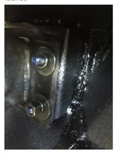
c. Attach the two included D-rings to the tabs on the front of the bumper.
