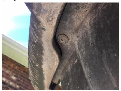
b. There are similar screws on the top of the bumper that need to be removed in the same way. This will free the plastic piece under the grill.
