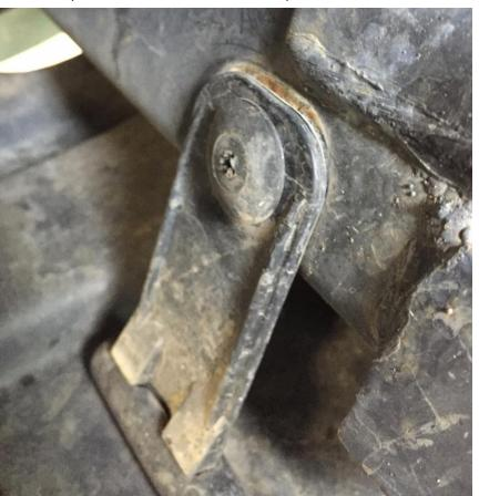
d. Using a philips screwdriver, remove the four screws on each fog light from behind the bumper and slide them out. You will not need them again later since you will use the included screws. Once removed these lights can be put aside until later by pinching and pulling out the orange plug shown below.
