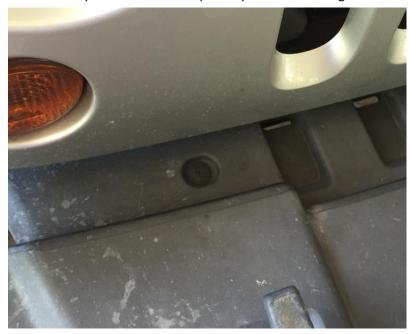
c. Two more pins are located behind the bumper that must also be removed
