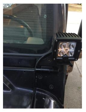
3. Connect lights to wiring harness and run harness into engine compartment. Connect yellow wire to positive battery terminal. Connect Black wire to automobile chassis. Ensure wire harness is not pinched or rubbing against sharp metal surfaces.
