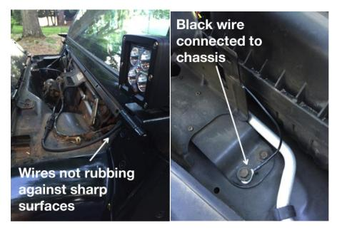
4. Run cables through firewall and behind dash. Mount switch into preferred location in dash and connect the RED wire to the switch terminal marked LOAD. Connect the YELLOW terminal to the switch marked SUPPLY. Attach the BROWN wire to the terminal marked EARTH. Attach the other end of the BROWN wire to a grounded metal surface behind the dash (usually a screw mounted to the firewall).
