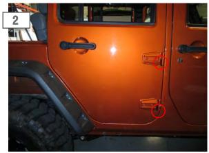
Locate the door hinge brackets and remove the hinge nuts(Torx T50) to allow the door to be removed.
