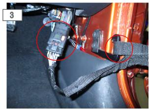
Disconnect the plug that supplies the door electric. Then remove the door strap.
