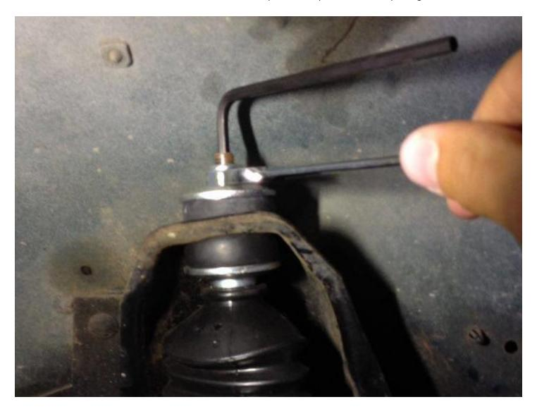
9. Another method commonly used to keep the piston rod from spinning in its bore, is to cut a rubber hose and attach it to the piston rod and hold it with channel lock pliers. I don't recommend this method because you don't want to chance bending the rod or damaging it and causing it to lose its seal and result in a leaking shock.
