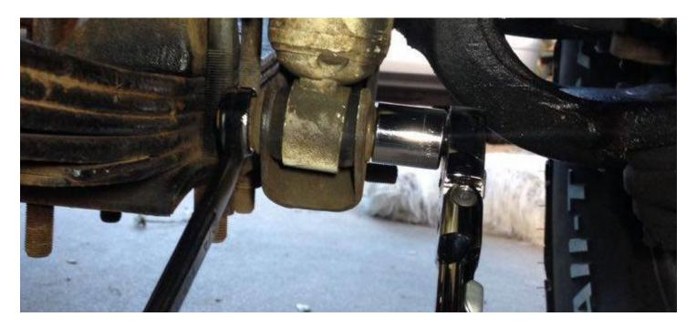
4. Now remove the old shock, it should slide right out. If it doesn't come out easy, pry it out with a screw driver. Before installing the new Bilstein shock, compare the compressed and decompressed length with the old shock to make sure they match up. Now for the next step you made need a friend to help compress the shock. I like to leave the green straps that came with the shock on until I'm ready to install the new shock.
