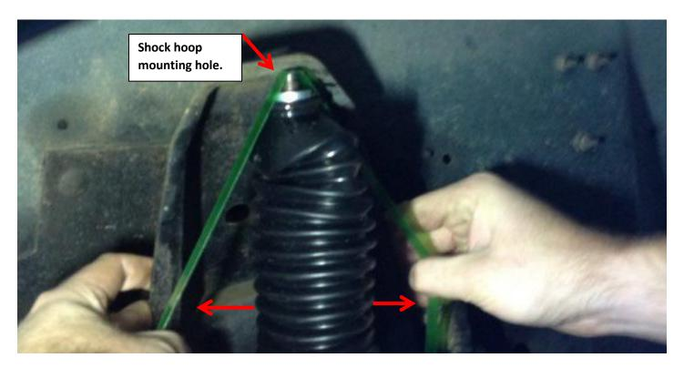
8. Reusing the old shock hardware (top nut), tighten down the top shock nut until the bushing fully seats on the shock hoop and you can see it compress slightly and it begins to flex outwards. The torque spec is 45 foot pounds. Use a 17mm wrench and an allen wrench. The allen wrench is used to stop the shock piston rod from spinning in its bore.
