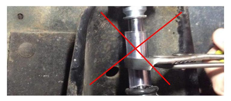
10. Installing the left front shock is the same as the right front; just don't forget to keep the washers and bushings facing the right direction. If the shock boots are bunched up from the way they were shipped in the box, just pull them down with your hand towards the bottom of the shock. They should straighten out.
