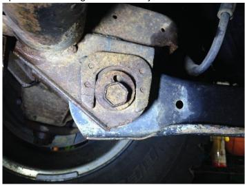
7. Support the front axle with a hydraulic jack. Remove shocks using a 13mm socket and wrench on the lower mounts, and a 15mm wrench at the stud. Use vice grips at the top of the stud or a strong clamp around the upper part of the shock to keep it from rotating. Save lower shock hardware.
