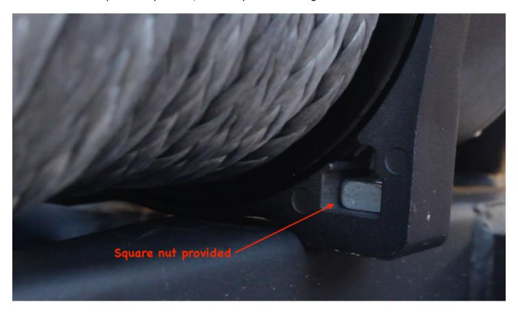
7. Using the 4 bolts provided, place a tightening washer on each and screw into the 4 square nuts from below the winch.
