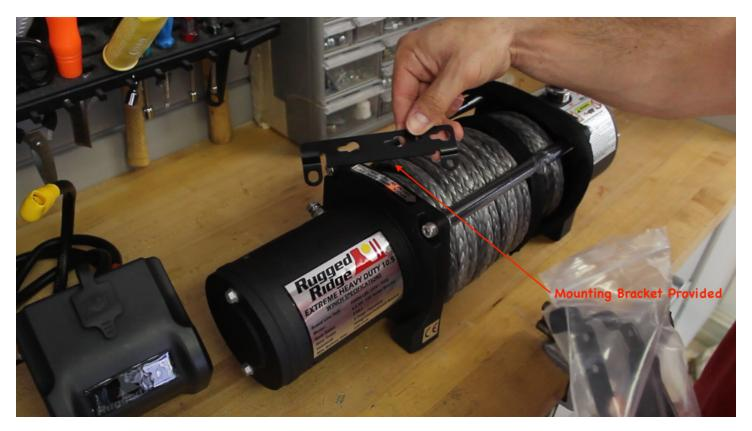
2. Remove the back left screw with allen key (Bolt 1)
