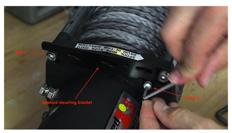
4. Secure solenoid onto solenoid mounting bracket with the 2 bolts on the left of the solenoid box.
