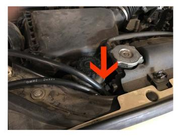
14. After you run your wires to the battery, make sure they're not going to snag anything in the engine compartment and connect the wires to the positive and negative battery terminals.
