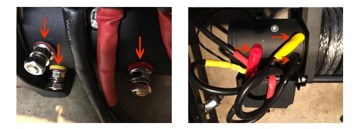
\*\*Before connecting any wires, be sure to slide the colored wire cover back behind the wire terminal connection\*\*
