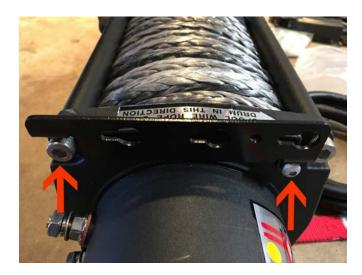
This is where you will mount the bracket before mounting the control box. You will use the existing bolt on the left and add a M5 bolt with M5 lock washer on the right side.
