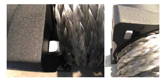
The trick here is to slide them all the way to the back of the winch and make sure they're seated properly. This way, they will be in perfect alignment when it's time to install the M8 bolts.
