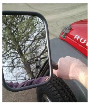
b) Rotate just the bushing so that the top or bottom of the bushing (the flat parts) are flush with your palm. From there, rotate the bushing to the nearest pair of holes on the arm.
