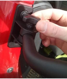
9. For each mirror, rotate and align the mirror as desired. Once aligned, use a phillips screwdriver to tighten the three screws on the reverse face of the mirror. This will help prevent the mirror from moving while driving. Do not over tighten these screws.
