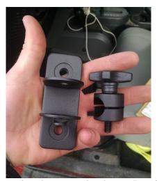
b) Install the mirror bracket using the proper hardware. Install with the welded nut on the lower side.
