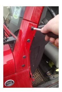
a) Using a socket wrench with a T40 bit can be helpful.
