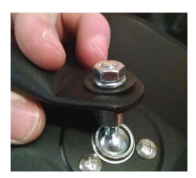
c) Tighten the assembly down, but don't over tighten.
