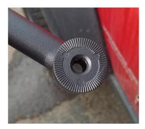
7. To align the passenger side bushing, repeat step 6 except hold the arm with your left hand.
