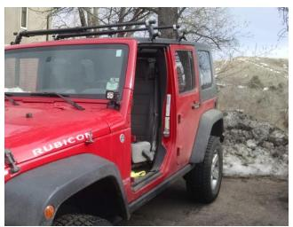
2. Using the T40 Torx screwdriver, remove the upper two bolts in windshield bracket located on the A-pillar.
