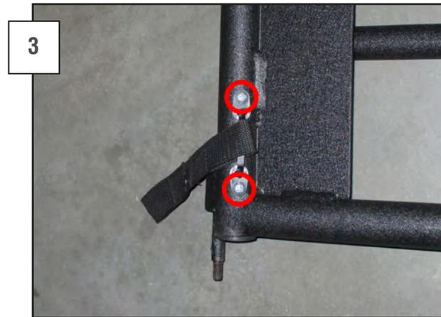
On the front, inner bottom of the door there are (2) screw holes. Insert the included strap mount through the included strap. Place the strap mount on the door and tighten down the (2) phillips head screws.
