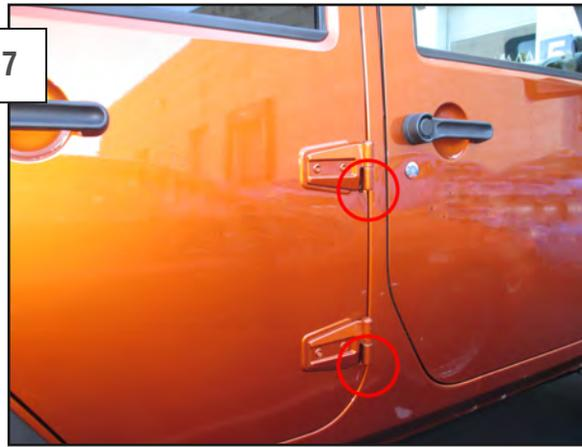
Using a T50 torx driver; Remove the hinge pin retaining nut from the bottom of the upper door hinge, then remove the lower hinge's retaining nut.
