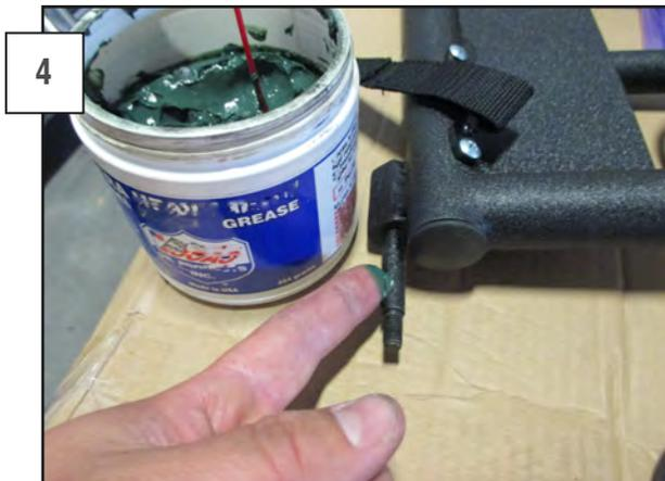
Lubricate the trail door's hinge pins with some automotive grease.
