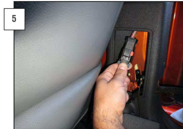
On the inside of the Jeep, behind the access door in the back. Remove the door electrical harness (is your vehicle is equipped). Push the red tab to the right, then press down on the locking tab and pull the harness apart.
