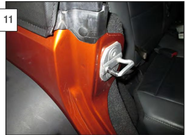
Some vehicles may have slightly twisted bodies or the strikers are worn from use. This may cause the doors to rattle lightly. Electrical tape can be wrapped around the striker to keep the doors from rattling.
