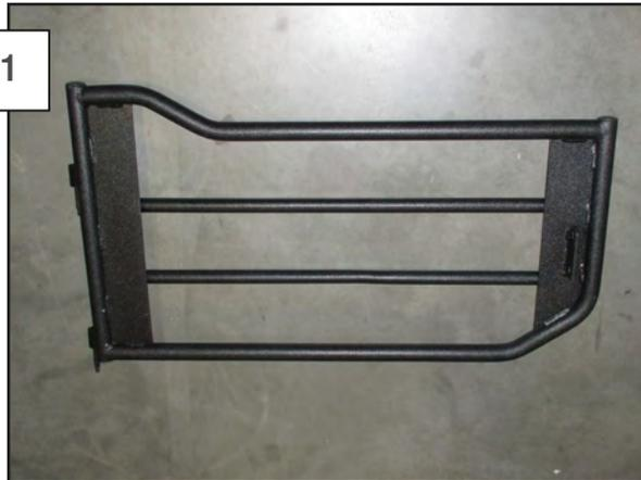
Lay the trail door on the ground, use a blanket between the door and the ground to keep the outside of the door from scratching.
