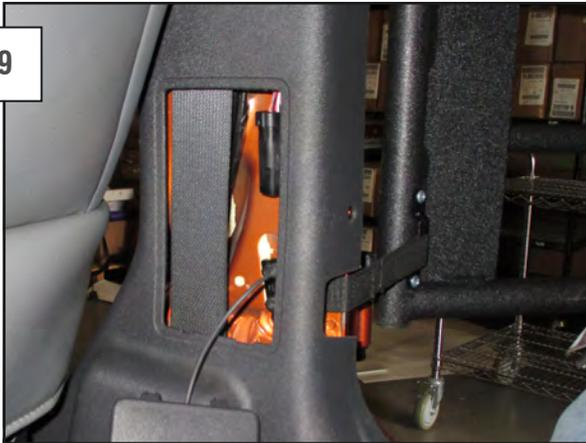
Place the strap over the top of the retaining hook and make sure the door is secured.
