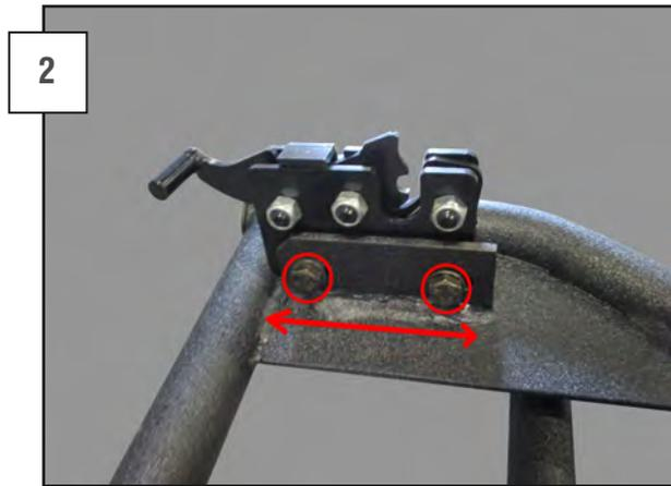
Install the latch, as shown, with the handle up top on the back side of the latch mount. Insert the bolts from the front of the door to the back of the door. Secure the bolts with the supplied nuts. Be sure to use a washer on both sides of the bolt and nut combination. Keep the latch loose so it can be moved up and down as needed, if it does not line up with the striker..
