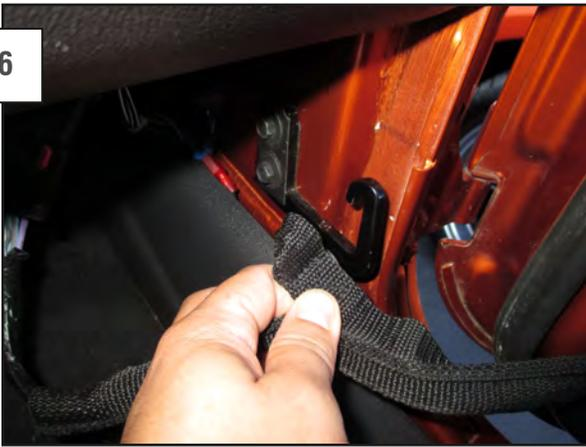
Next to the electrical connector is the door securing strap. Pull this up and over the vehicle's strap retaining hook. CAUTION: Make sure you keep the door supported from here on out. The door can swing wide open and dent the fender without this strap.
