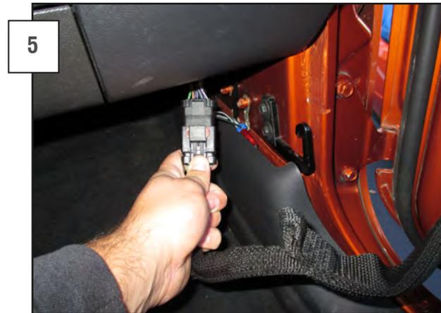
On the inside of the Jeep, Under the dashboard. Remove the door electrical harness (is your vehicle is equipped). Push the red tab to the right, then press down on the locking tab and pull the harness apart.
