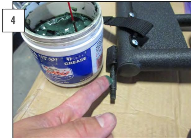
Lubricate the trail door's hinge pins with some automotive grease.
