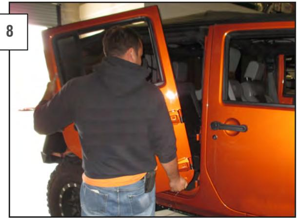
Remove the door by grasping it securely and lifting straight up, then pulling it away from the vehicle. The doors can be heavy and it may be necessary to have someone help with the uninstall. If the door is too hard to remove, it can be swung back and forth slowly to aid in removal.
