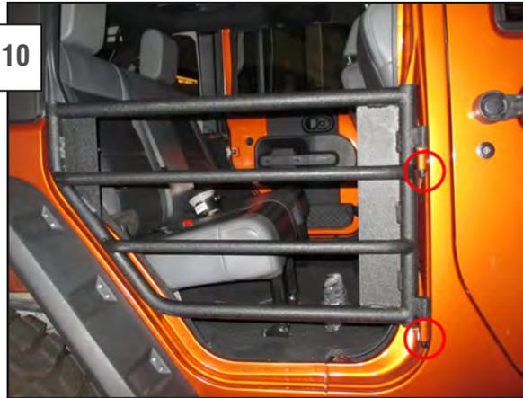
Install the included washer, lock washer and nut to the top hinge, install the other set on the lower hinge. Tighten the hardware with a 13mm socket. If the door creaks or is hard to swing, loosen the 13mm nut until it swings freely, yet is still secure. Close the latch on the striker and tighten down the hardware to keep the latch in place.
