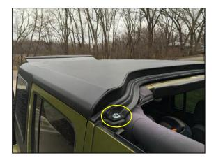
6. Place front section onto Jeep and secure with four interior clamps. Take care not to over-tighten:
