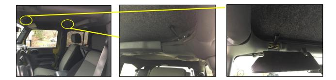
7. Place the drip protectors on inside corner of each rear door frame:
