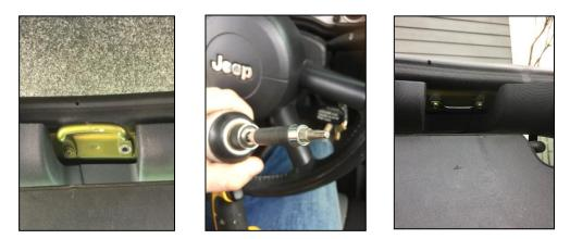
4. Place main top section onto Jeep and bolt down with six (6) 13mm bolts (3 per side) with washers and nuts (supplied):
