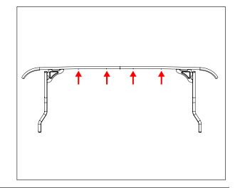
3. Flip soft-top fabric towards the front of the vehicle to expose the C-Pillar bow.
