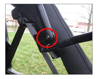
9. For 2007-2009 model year, remove the bar ends from the soft-top tubes . There is a small self tapping set screw that must be removed first. Insert the spacers onto the bar end and reinstall into the tube. Screw the set screw back in into the tube.
