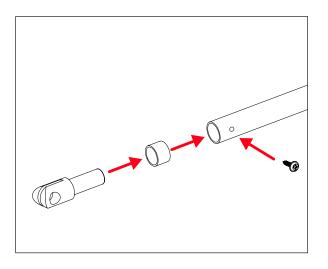
9. Attach Left-Hand arm to the Left-Hand assembly using the supplied M8 flat head bolts. Repeat for right side with right-hand assembly and right arm.
