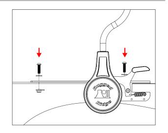
13. Attach bow to the left and right arms using the supplied M8 button head bolts and lock nuts.
