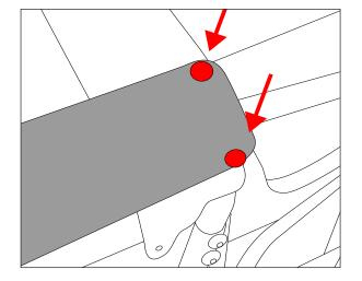
16. Fold soft-top back into correct position and attach the fabric to the spring assist bow and rearmost bows the same way as they were removed in steps 2 and 6 using the supplied self-tapping screws.
