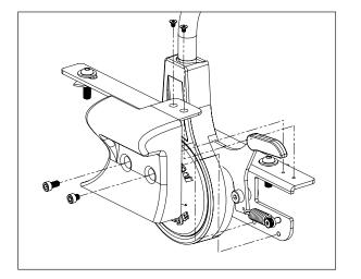
11. Install Left-Hand assembly to the body tub using M8 button head bolts, washers, and nut plates. Repeat for the right-hand side.
