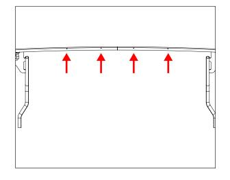
6. On 2010-2012 model year vehicles, remove the fabric cover and disconnect the soft-top's cable by unhooking the spring.
