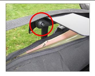
15. Using the supplied self tapping bolts. Secure the nylon support strap to the sides of the bow. The bow has pilot holes already drilled in the correct locations. However new holes will have to be made into the nylon support strap. Use a punch to create pilot holes into the strap.
