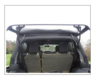
4. Drill out rivets attaching nylon support strap to bows using a 1/8" bit.
