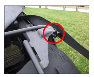
7. Disconnect the C-Pillar bow from the tube ends using a T-27 Torx bit. Retain factory fastener which will be reused in step 14.
