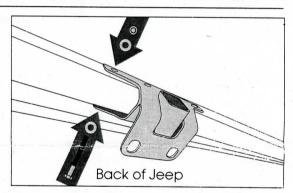
2. Insert trailer wiring, if equipped, into the trailer wiring mounting tab. Installation is now complete.
