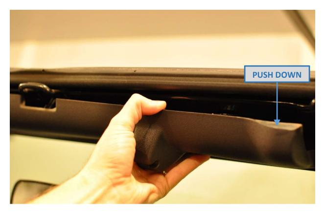
5. Remove the footman loop. For 2007-2010 model JK's (shown in picture), it will be necessary to drill out the 2 rivets using a 3/8" drill bit. For 2011 and new models, simply remove the 2 Torx screws.
