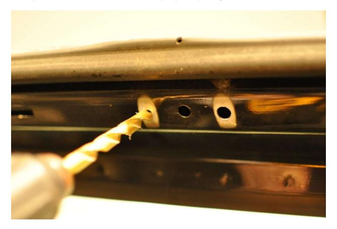
7. Insert the 2 rubber well nuts into the newly drilled 3/8" holes. If well nuts do not fit snugly in the holes, a small amount of glue can be used to hold them in place.
