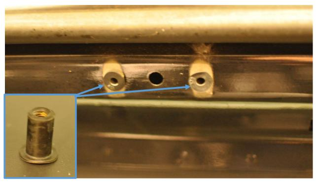
8. For 2007-2010 model JK's (shown in picture) use the provided 5 x 20mm screws to install the CB mount with the footman loop sandwiched between the windshield frame and CB mount. For 2011 and newer model JK's use the factory Torx screws to install the CB mount with the footman loop sandwiched between the windshield frame and CB mount.
