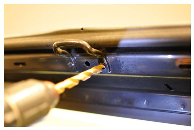
6. For 2007-2010 model JK's it is necessary to drill out the 2 footman loop holes in the windshield channel to 3/8" to accept well nuts. Be careful to not drill too deep or you may damage the exterior of the windshield frame.
