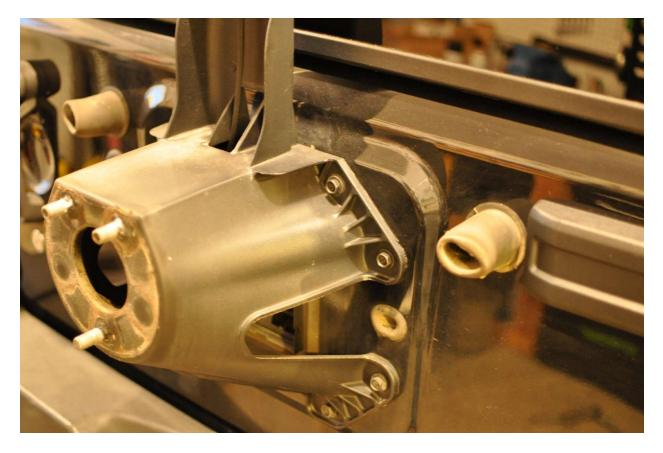
2. Remove the 2 upper right 8mm bolts using a 13mm socket
