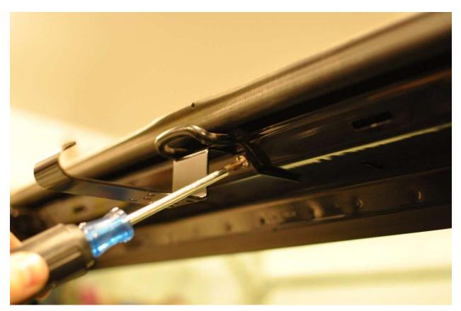
9. Remove the center positioning lug from the plastic windshield frame covers using a diagonal cutting pliers or similar. This is necessary because the new CB Radio Mount covers this hole in the windshield channel.
