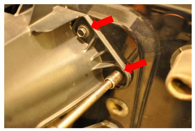
3. Install the CB Antenna Mount using the 2 supplied 8 x 40mm hex bolts, lock washers and flat washers. Torque the bolts to approximately 10 ft-lbs. Note that the CB Antenna can be installed in either hole of the bracket. Remount the spare tire after installation of the CB Antenna is completed.
