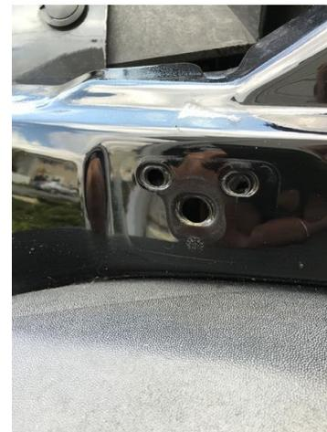
5. Attach the new top bracket using the hardware provided. Tighten into position with the 4mm hex socket and 10mm socket. Ensure to use the (2) flat washers also supplied with the kit.
