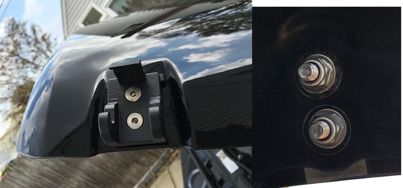
6. Position and align the bottom bracket. Pay close attention to the alignment tabs and the holes on the fender. Secure into position with the 4mm hex and 13mm sockets. Note: You might have to disassemble the bottom bracket in order to access the mounting bolt. To remove the mounting pin, using the 5mm hex socket and 5mm allen key. Once mounted, attach the hoof bump stop onto the top mounting tab.
