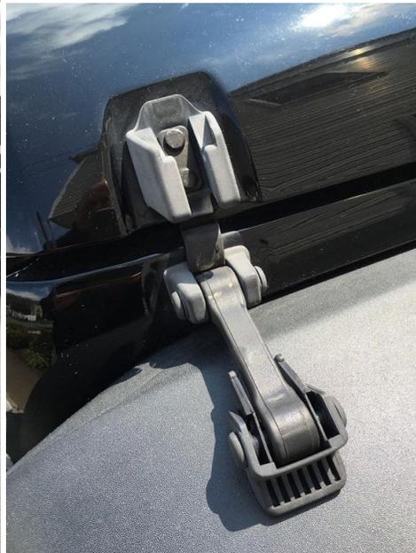
2. Using the flat head screw driver, pry off the cap end of the center factory pin.
