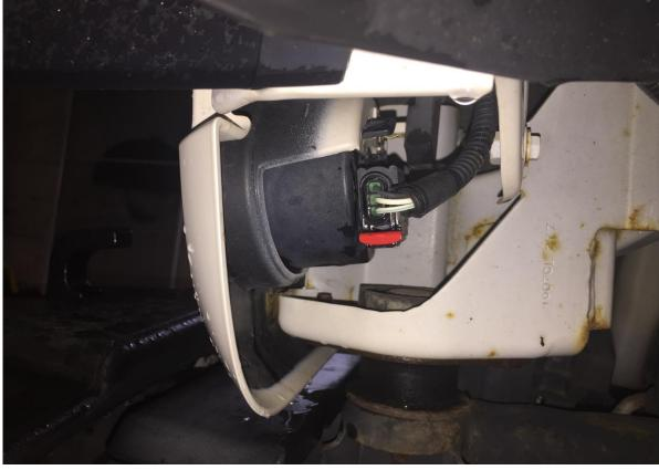
4. Remove grill from vehicle careful to not break bottom retainer clips
