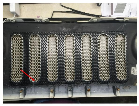
6. Place support brackets across insert and mark where holes are to be drilled (make sure the brackets are tight enough that any bend in grill after reinstallation will not loosen them) repeat for other side
