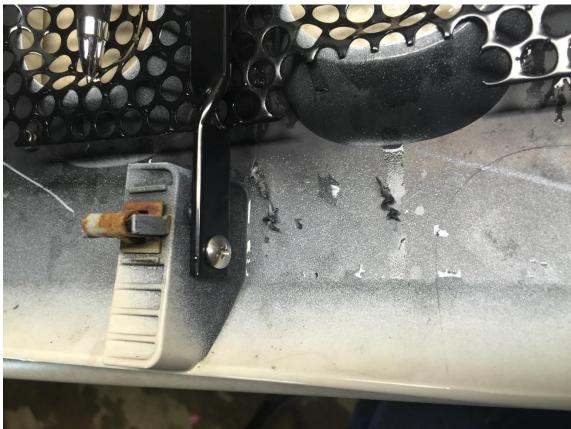
8. Reinstall grill onto vehicle, make sure all retainers at bottom of the grill and by fog lights are firmly seated and reinstall retainer clips along top of grill (This will require getting a little rough and forcing the grill back into place due to the brackets being slightly in the way)
