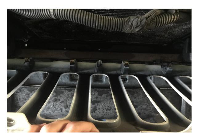
5. Lay grill on flat surface and place mesh grill insert with cutout on bottom drivers side
