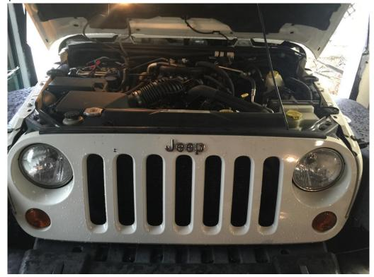
2. Locate and remove 6 panel retainer clips (in my case they were required the use of a Philips head screwdriver to remove the center and they were striped, 4 on top of grill and 2 on the sides near headlights)
