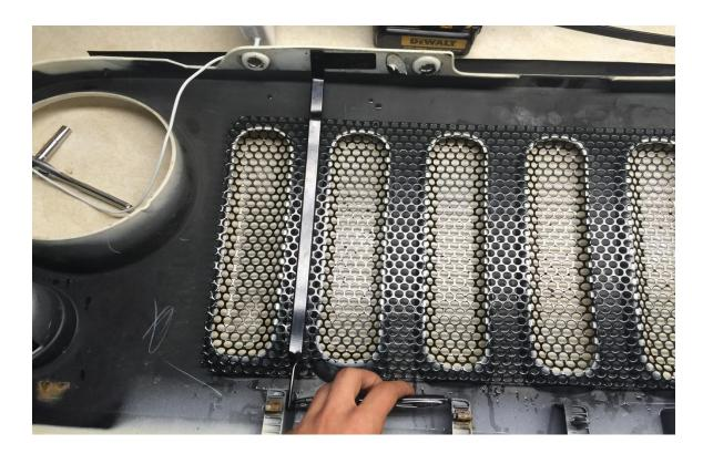
7. Insert bolts through drilled holes and brackets placing washer under the nut and tighten down with 9/32 socket repeat for other 3 holes (I recommend install the bolts on the top of the grill with the nut facing up and the head facing down to allow easier installation back into vehicle
