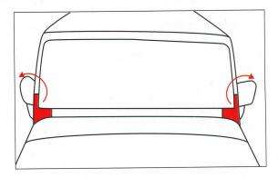
4. Install assembly to vehicle using factory hardware retained from Step 1. Adjust fitment if necessary and securely tighten all bolts.
