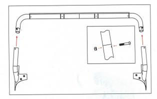
3. Remove the factory LH and RH brackets. Retain factory hardware for later use.
