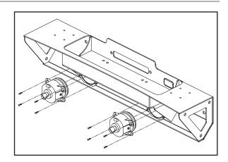
5. Install bumper ends using (3) 12mm washers and (3) 12mm lock nuts per side. Once all nuts have been started tighten nuts securely.
