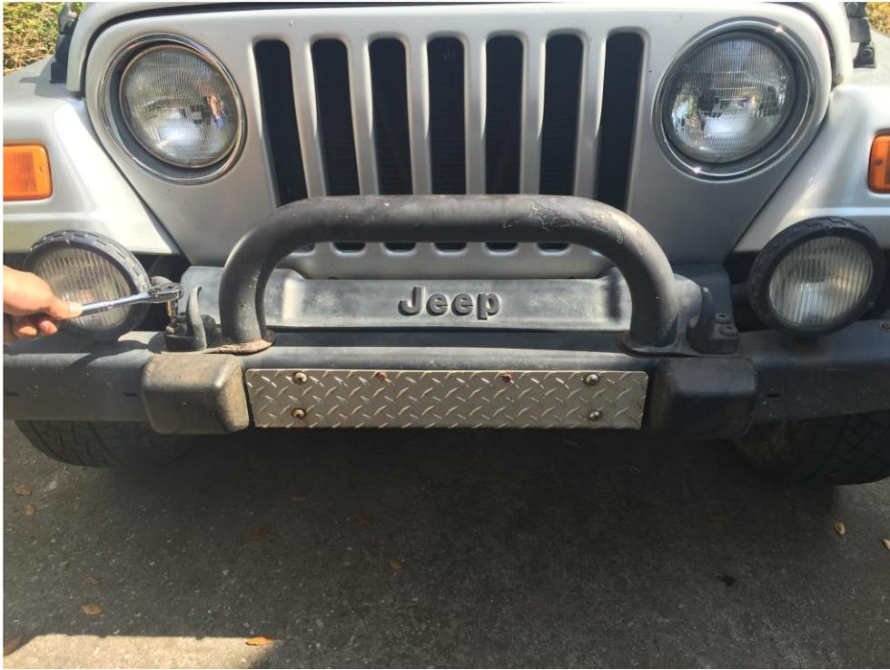
3. On both sides of the sway bar cover, remove the 10mm bolts and pull the cover away from the vehicle. This will give you extra room to work
