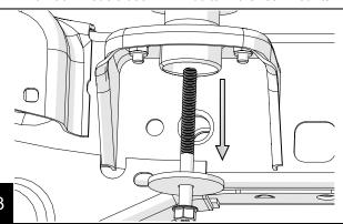
Place a floor jack under the right side of the body with the lift plate below the section of body just outboard of the frame, as shown. Place a block (2x4 or a 4x4) on the jack to distribute the load of the body.
