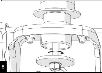
On the front right mount, **loosely thread** one of the supplied custom nuts onto the stud in the center of the body mount hole.
