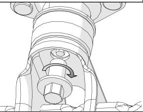
Lower the right side of the vehicle body completely onto the new body mounts.
