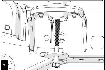
**Loosely thread** the new bolts with washers supplied in the kit through the body mounts and into the body of the Jeep.
