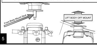
Slide the TeraFlex spacers into place.
