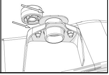
Lower the right side of the vehicle body down far enough to thread the supplied bolts into the body mount holes.
