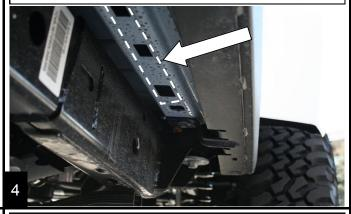
Raise the right side of the jeep body enough to insert the TeraFlex body lift spacers between the body and the factory mounts. It may be necessary to re-position the jack along the body as you progress from the front of the vehicle to the rear. You will need to raise the body enough to fit a spacer between the stud of the forward-most mount and the frame.
