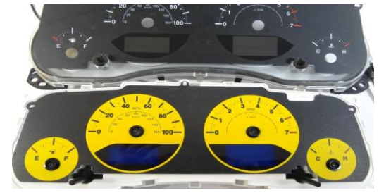
19. Place the new US Speedo gauge face into position. Replace the trim circles.
