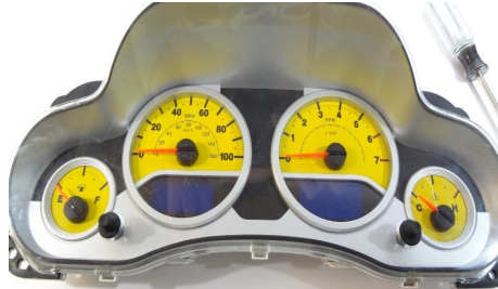
22. After each needle is correct, put the lens on and install.
