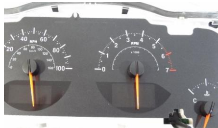
14. Twist each needle down past zero or the low stop.
