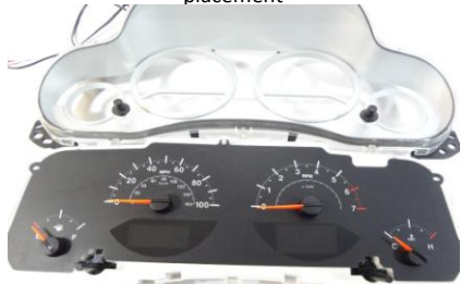
13. Make sure to mark the needle position or take a pic.
