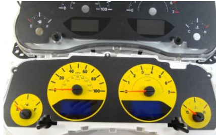
21. Set each needle. Plug into the car and check.
