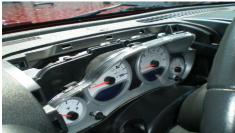
4. There are 4 screw holding cluster in place.
