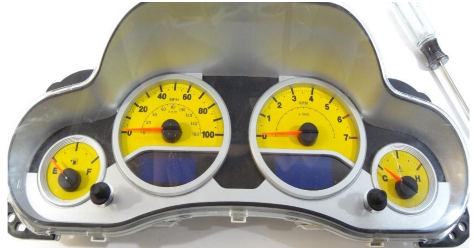
22. After each needle is correct, put the lens on and install.
