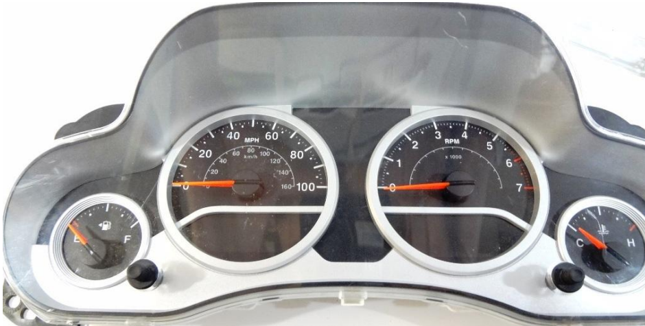
20. Set each needle as the picture you took. Use the handle as a height guide under the needle hub
