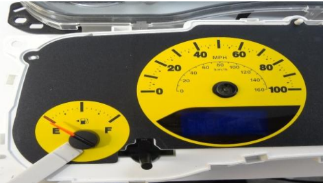
20. Set each needle as the picture you took. Use the handle as a height guide under the needle hub
