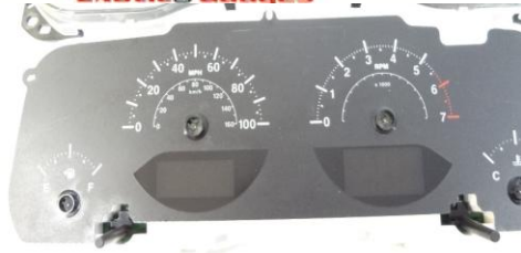
16. After the needles are removed, remove the black plastic circles. KEEP.
