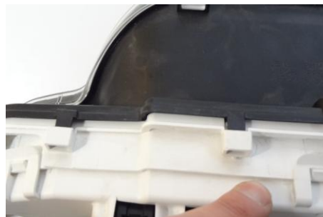
10. Press to release the tabs to remove the lens and top trim.
