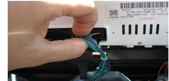
7. Push down on the tab to release the plug.
