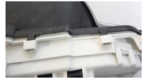
11. It is tricky to get several to release at the same time.
