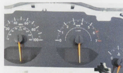
14. Twist each needle down past zero or the low stop.
