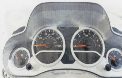
9. Take cluster into a clean area to install the gauge face. Take a pic of the needles placement
