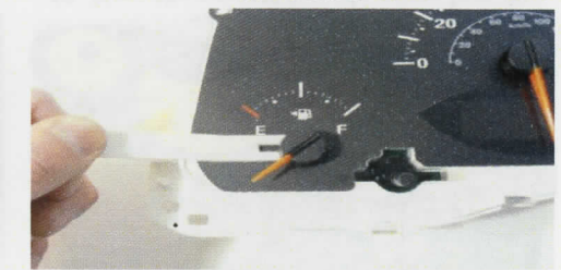
15. Use the needle tool to remove each needle. Pull straight up.
