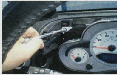
5. Remove the 4 screws.
