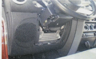
1. Pull down trim under steering wheel.
