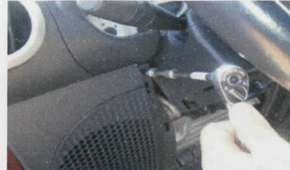
2. Remove 2 screws from the top trim.
