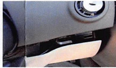
2. Pull down the lower trim panel. Only held in with snaps.
