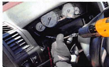
5. Remove the screws holding the speedometer in place.
