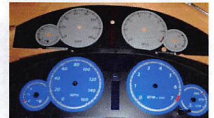
15. Put the new gauge face in place.
