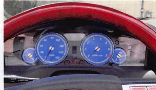
18. Check the needle placements before the completely installing the cluster.
