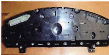
9. Remove the screws on the back of the cluster to remove the lens.
