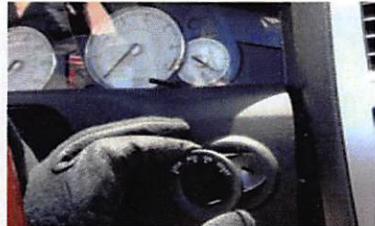
1. With a small screw driver, snap out the key ring.
