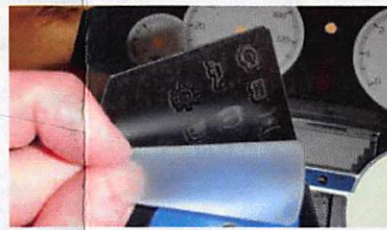
14. On the back of the new gauge face is a plastic liner, remove.
