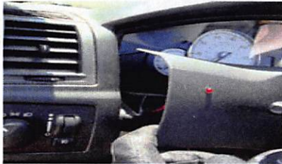
4. Pull off the trim under the speedometer.
