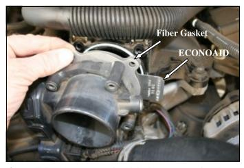
**3.** Install the ECONOAID Throttlebody Booster against the intake manifold with the logo facing the throttlebody. Next install the supplied gasket between the ECONOAID and the throttlebody.
