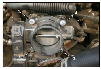
**4.** Reinstall the factory bolts and tighten them in a cross pattern to the manufacturer's specifications. Before starting the engine, open and close the throttlebody to make sure there are no obstructions.
