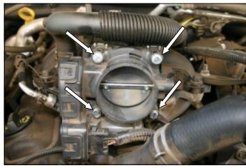
**2.** Remove the four bolts that hold the throttlebody to the intake manifold.
