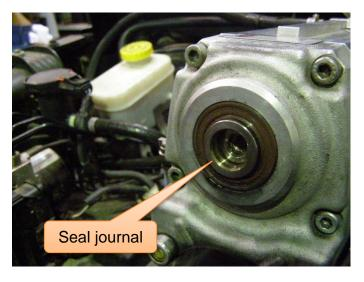
If the seal journal is removed accidentally from the supercharger, apply a layer of high temperature lubrication grease in between the lips of the lipseal. Insert the seal journal into the lipseal locating the spigot on the supercharger drive system.
