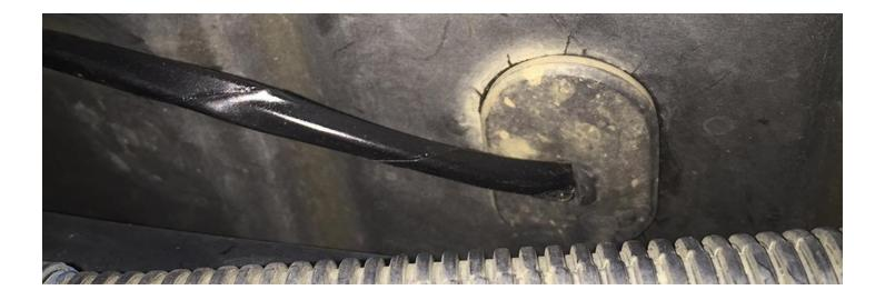
3. Once all wiring is run through passenger floor plug and into the passenger interior compartment plug all wiring into adapter.
