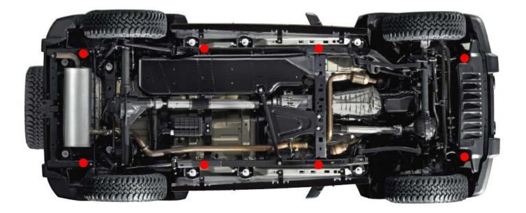
2. Install Rock Lights and run all wiring to the passenger side undercarriage. Option: Use magnets with some Gorilla glue to help secure if you don't use the wire clips.
