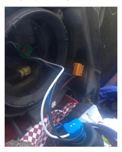
9. Install HALO headlight with o-ring, metal mounting ring (from removal step 3) and torx screws.
