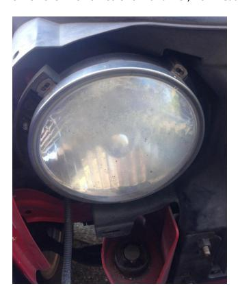
4. Remove headlamp and metal mounting ring (keep metal ring) Maintenance Tip: Clean/Buff metal ring.
