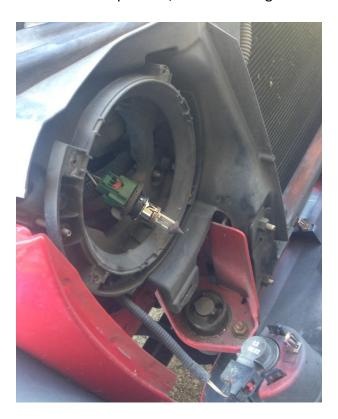
5. Plug HALO headlight into factory wiring harness.
