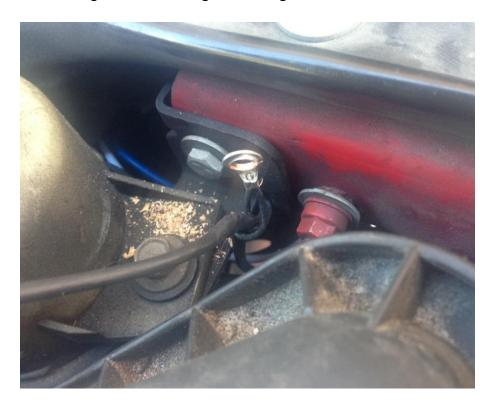
Maintenance/Adjustment Tip (optional): Use Drill and drill bit to increase wire connection so that it fits onto ground.
