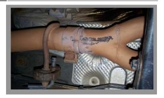
Loosen the clamp at the factory Y-Pipe. Remove the rubber grommets holding the exhaust. Loosen the connection at the head pipe and muffler, then remove the head pipe and let the muffler hang out of the way. <u>NOTE!!!</u> Be sure to use lubricant to aid the removal of the rubber grommets and muffler.
