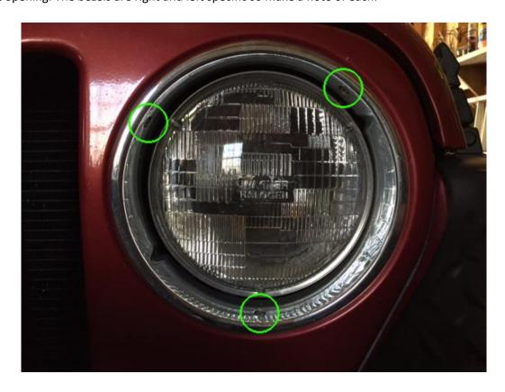
2. Using a T15 Torx driver, remove the four (4) screws from the headlight retaining ring. The retaining rings are right and left specific so make a note of each.
