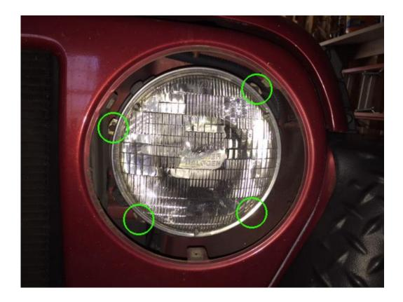
3. Reach behind the headlight and disconnect the wiring harness.
