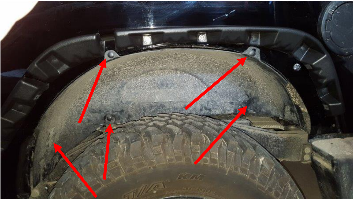
29. You may also need to trim the top edge of the rear upper mounting tab
