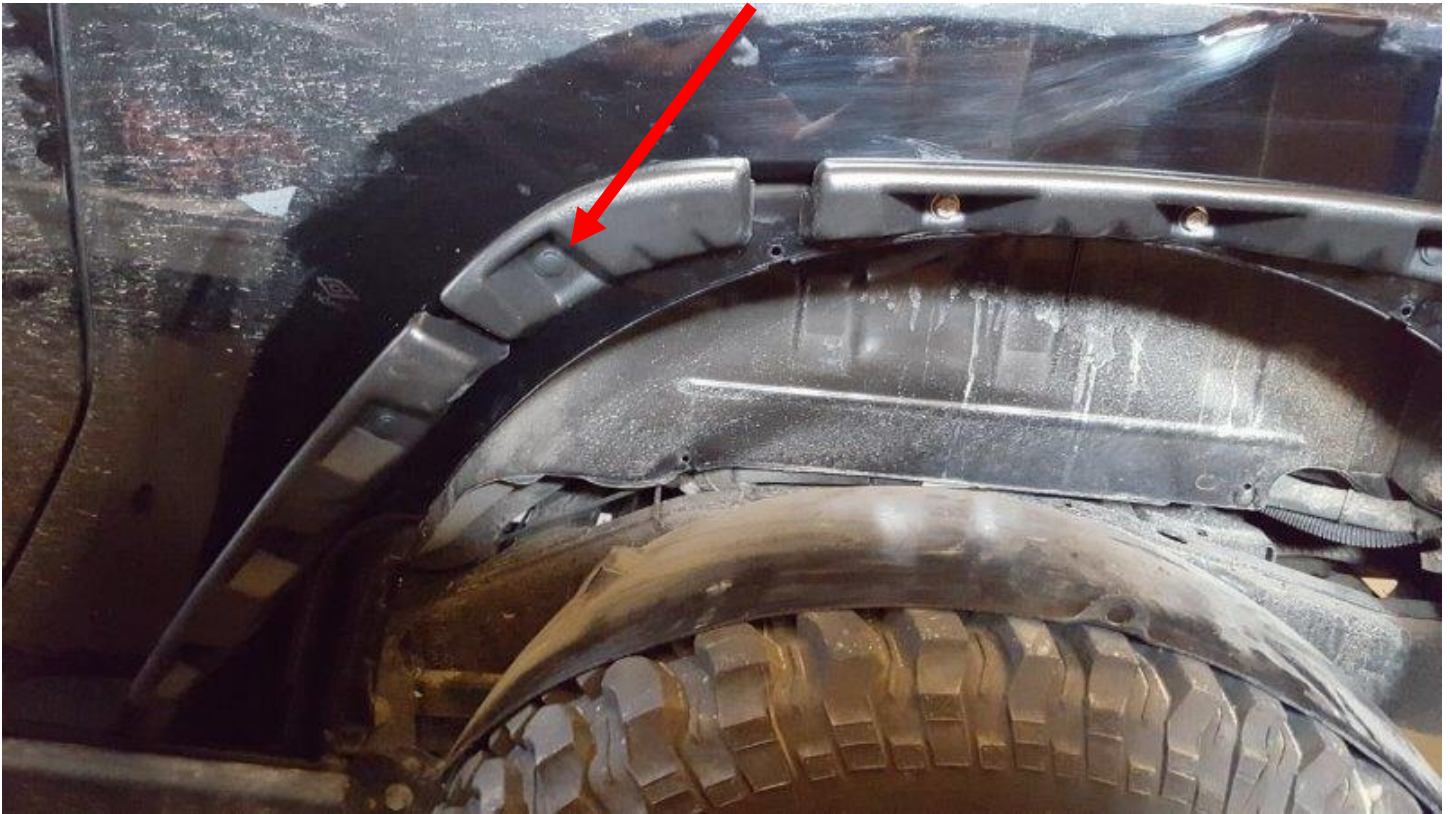
28. Next, reinstall the trimmed splash guard using 5 supplied push retainers
