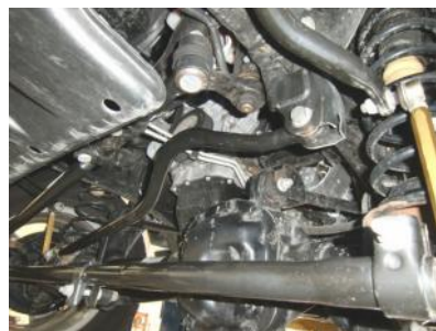
2. With the vehicle properly supported locate the front track bar.
