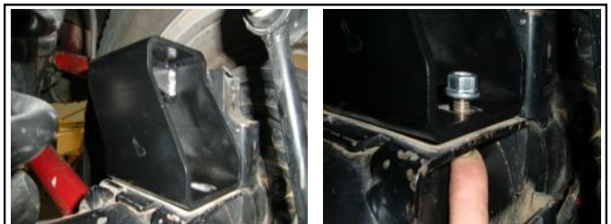
24. Install new bump with supplied hardware. Bump stop pad should be leaning towards front of vehicle.
