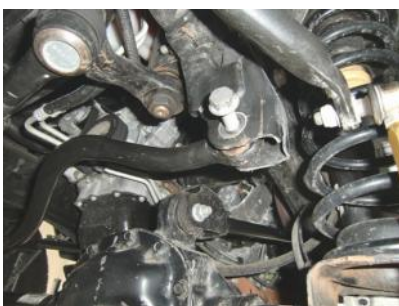
3. Remove the track bar from the frame.
