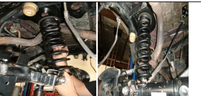
25. Install new coil with factory rubber boot on top.
