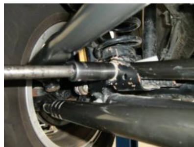
4. Next, unbolt the track bar from the axle and remove from vehicle.
