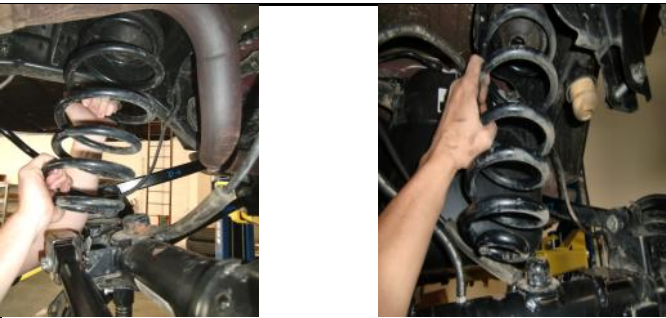
23. Lower the rear axle and remove the springs.
