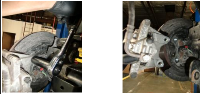
21. Unbolt and remove rear brake caliper and hang caliper out of the way.
