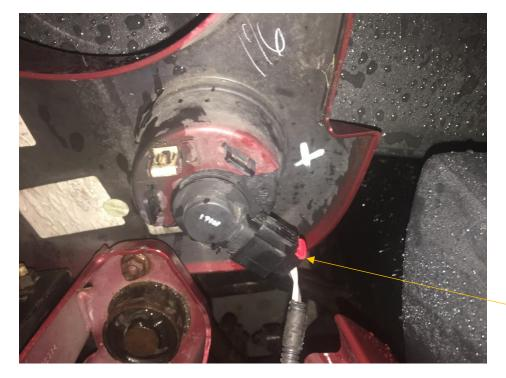
5. Press the clips holding the turn signal housing inward so that the housing can slide out of the grille.
