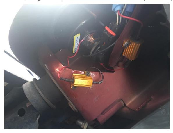
21. Here is the completed left hand side, where the two resistors are attached to metal parts of the Jeep.
