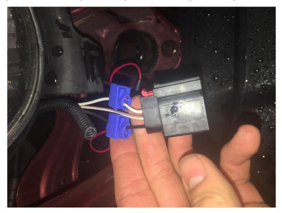
16. You can now attach the headlight assembly to the grille. There is one more resistor that must be connected to the tap connector of the ground wire. Here you can see that the resistor coming out of the headlight itself must be attached to the tap connector of the ground wire (Pointed to with the yellow arrow). NOTE: Electrical tape must be put around the tap connector to ensure that the resistor wire does not come out of the tap connector.
