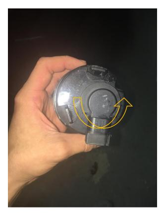
7. Then remove the factory halogen lightbulb from this piece.
