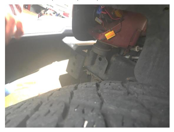
20. Here is the completed right hand side, where the two resistors are attached to metal parts of the Jeep.
