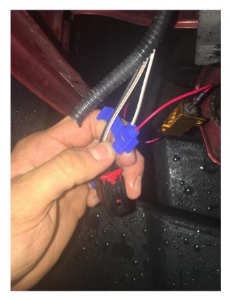
13. Push down on the metal part of the tap connector with pliers so that both wires are punctured by this metal piece and are in the tap connector snugly. Then close the tap connector with the piece that goes over the metal piece.
