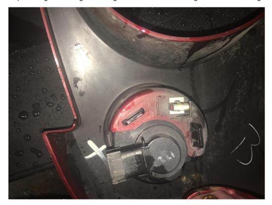
6. With the turn signal housing out of the grill, turn counterclockwise on the piece which holds the light to the outside housing.
