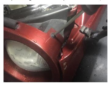
3. Do not try to pull the grille right off the Jeep because the turn signal wiring must first be detached.
