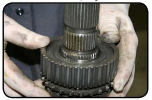
19. Install the new short shaft with the front output shaft and the drive chain.
