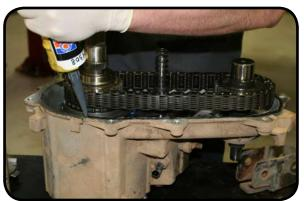
21. Install the rear half of the case. Make sure that the oil pick up is installed into the pump and the magnet is installed in the case. While installing the rear case slide the oil pump onto the shaft. Torque the bolts to 25 ft-lbs.
