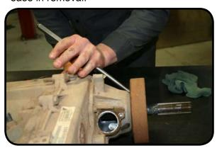
8. Remove the rear output shaft seal.
