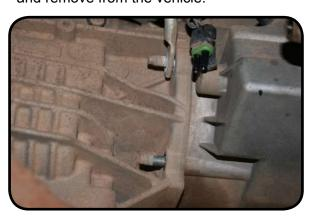
6. Remove the slip yoke boot using a flat head screwdriver to loosen the clamp.
