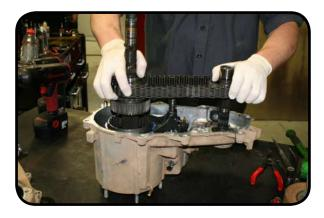
14. Remove the drive sprocket snap ring and remove the drive gear from the main shaft.
