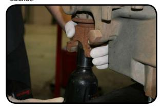
10. Place the transfer case onto the mounting studs. Remove the rear output shaft snap ring.
