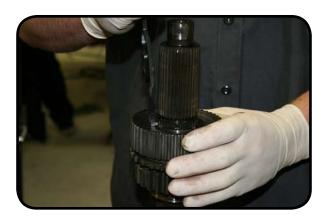
15. Check the mode fork inserts for damage. If they are worn replace them with factory replacement parts. Remember which way the synchro sleeve goes on the range fork. The short half of the splines should go down.
