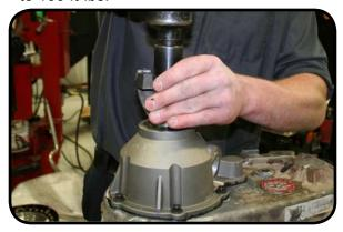
25. Reinstall the speed sensor into the transfer case. To make sure that the gears are engaged by rotating the yoke and putting your hand on the speed sensor. You will be able to feel the speed sensor gear turn. Install the speed sensor clamp and bolt and torque to 8 Ft-lbs.
