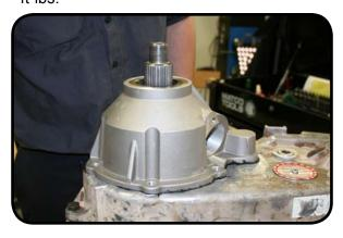
24. Install the new yoke. Use silicone adhesive on the splines of the yoke to create the seal. Use red thread locker on the yoke nut and torque to 100 ft-lbs.
