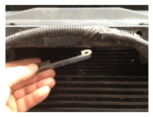
Insert the fixture from the side as shown, into the steel structure opening. Note; Match the fixture rotation to the photo as this will position the fixture forward into the opening and allow the 3 edges to line up.
