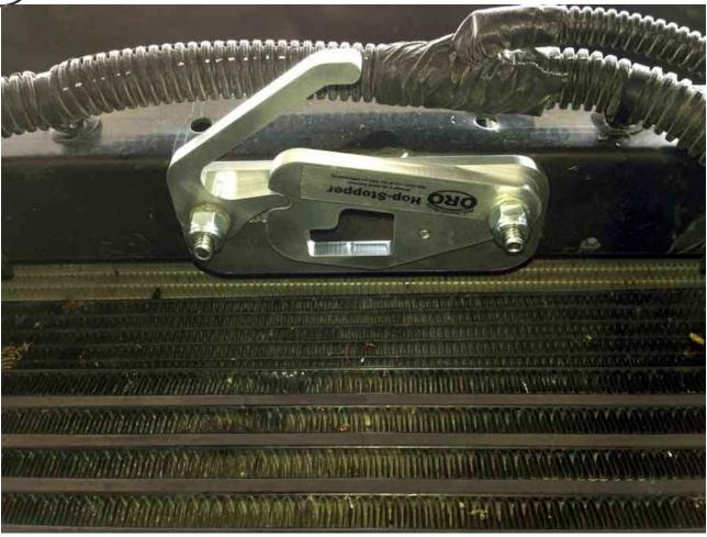
Unlatched, the roll pin will prevent the lever from opening past this position. Make sure that whenever your hood is open, you have the lever in this position. Closing the hood with the lever in the latched (Closed) position may cause the hood to push the moving latch mechanism downward enough to prevent the latch from grabbing the hook and closing.
