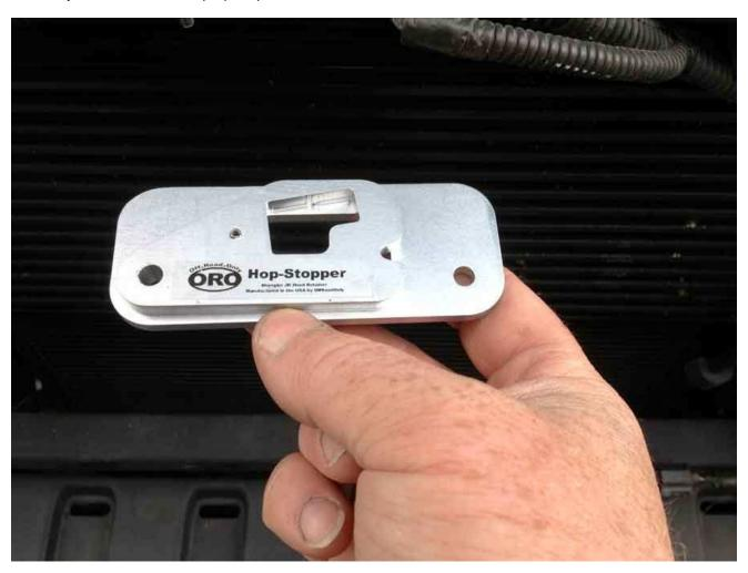
With these two parts positioned as shown, with the roll pin in the small slot in the larger square base, you are ready to invert these 2 parts and pass them over the 2 machine screws. The left side, as shown, will slide on the drivers side machine screw while the base slides over both screws at the same time. Install the lock washer and lock nut to hold the parts in place.
