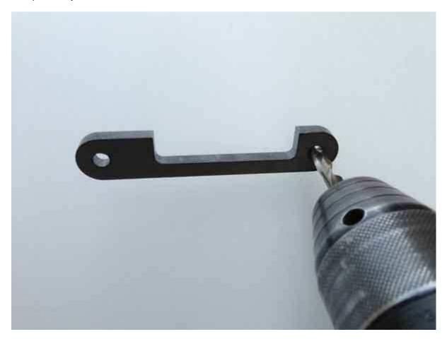
Now, there are 2 holes,  $\frac{1}{4}$ " in diameter, to either side of the square opening for the hood hook. We are going to use these 2 holes on the top of the steel structure. The raw steel piece included in the kit will be inserted inside the steel structure from the bottom as shown. When positioned properly, with the cut out in the raw steel fixture will match the opening on the bottom of the steel structure and the 2  $\frac{1}{4}$ " holes will be directly below the upper holes.
