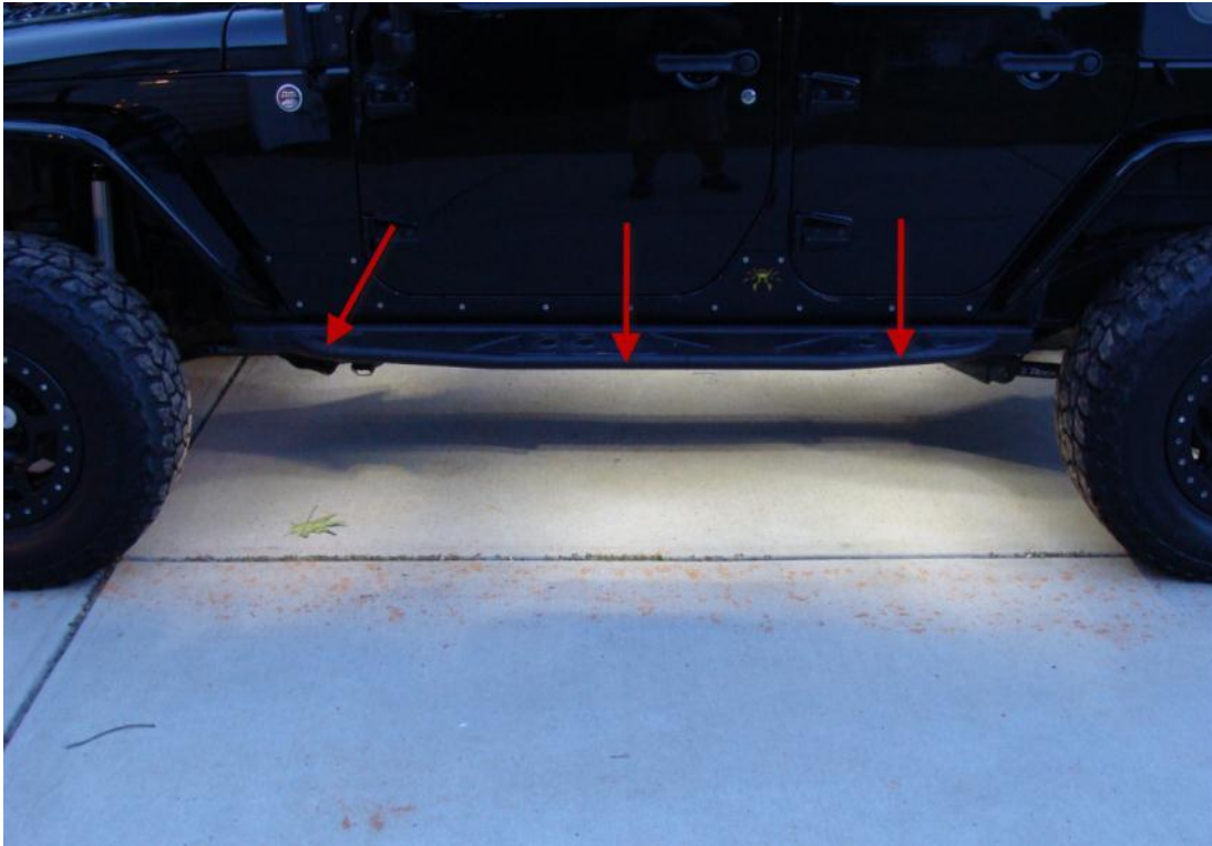
FIGURE 3 – LiteSPOTs placement on example vehicle
