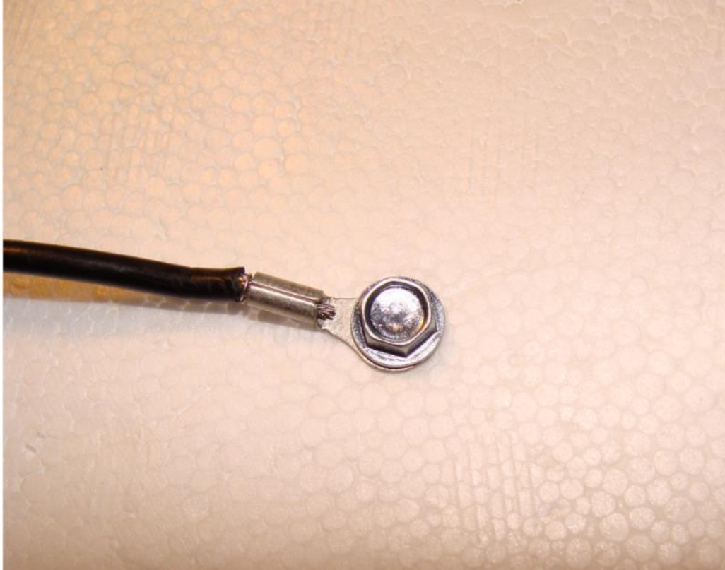
Figure 11 – BLACK 20g wire GROUND connected to vehicle body/frame
