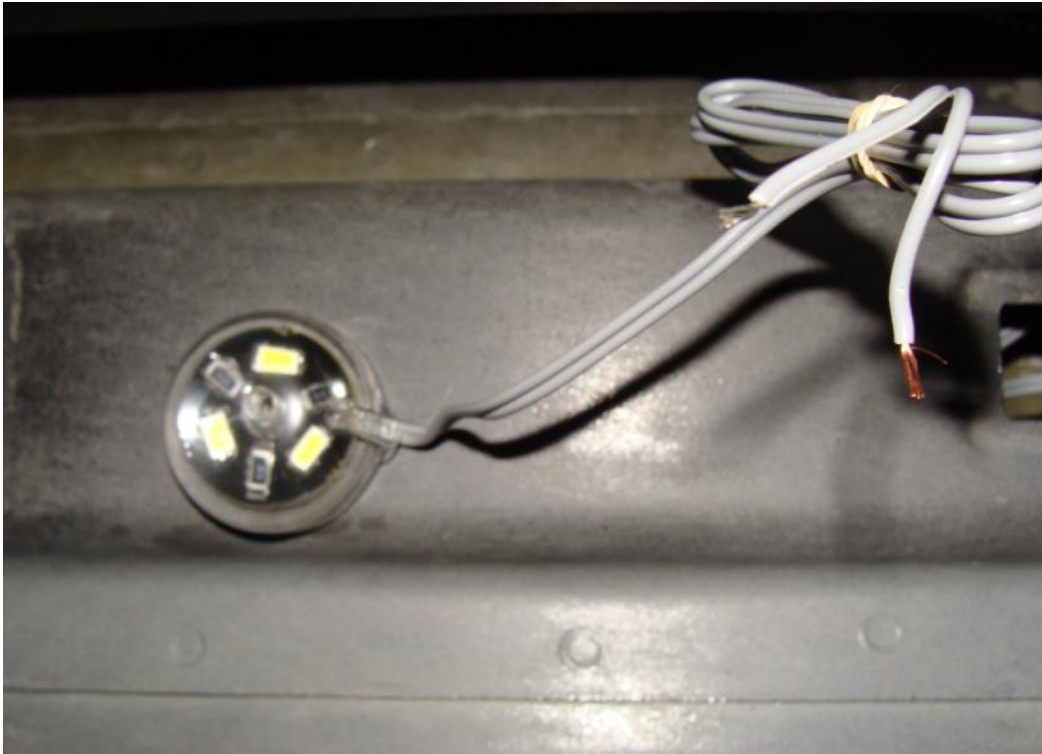
Figure 15 – Wired LiteSPOTs pod and wires secured using zip tie
