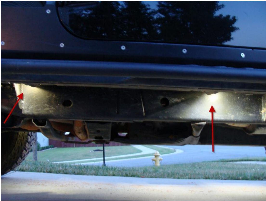
FIGURE 4 – LiteSPOTs placement under vehicle
