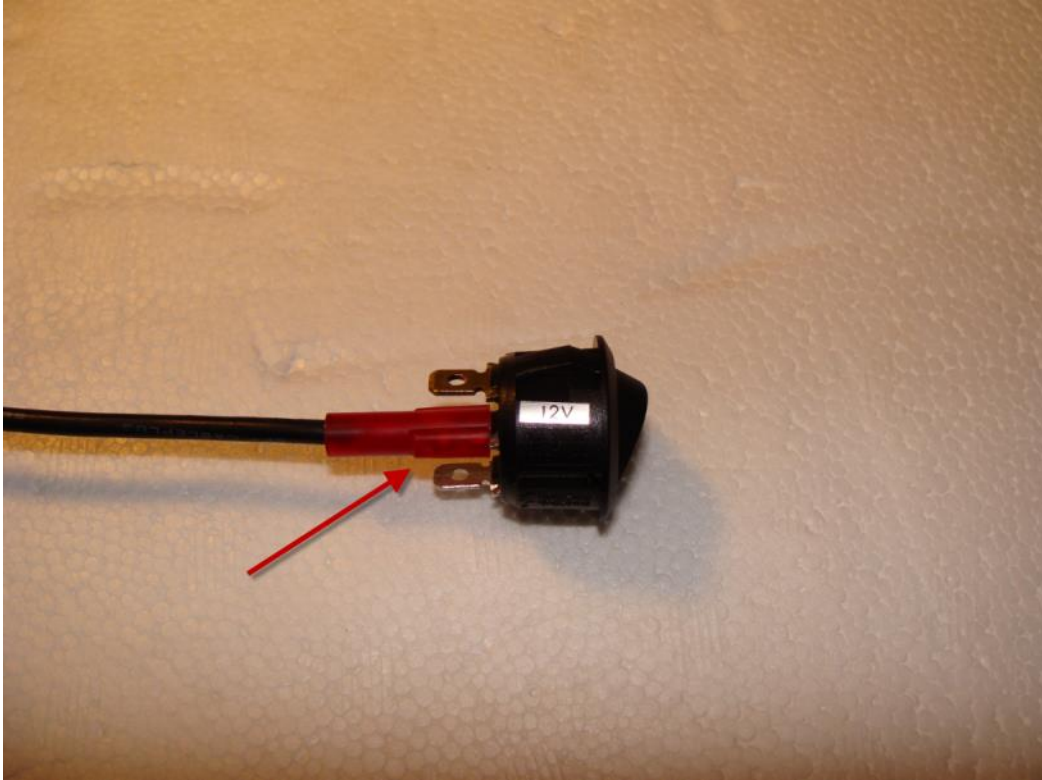
Figure 12 – BLACK 20g wire connected to Terminal 2
