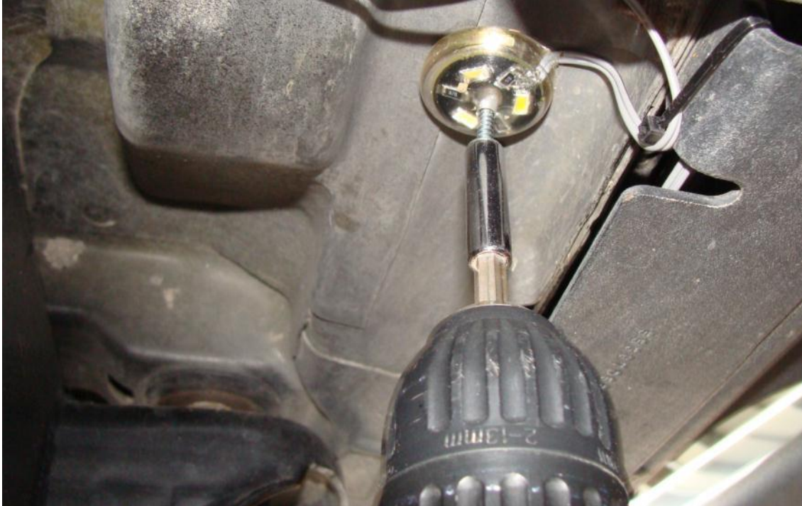
Figure 16 – Securing LiteSPOTS pod using self-tapping screw
