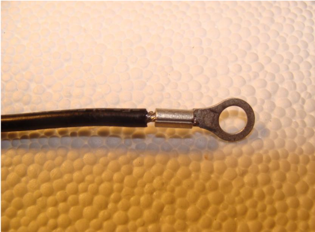
Figure 5 – Flat round terminal on 20g BLACK (POSITIVE) wire
