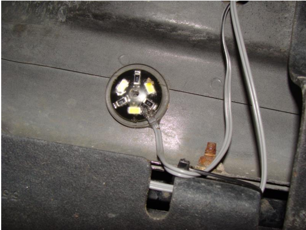
Figure 15 – Wired LiteSPOTs pod and wires secured using zip tie
