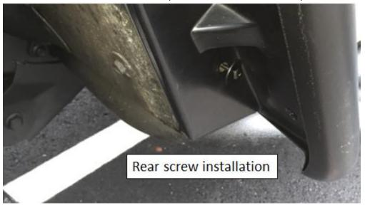
b. Now install screws in the remaining 5 positions. Install each screw by using the supplied flange nuts on the interior of the rear fender well. Using a washer between the screw head and fender flare, fasten each screw hand tight, ensuring you do not apply too much pressure and crack the plastic flare.
