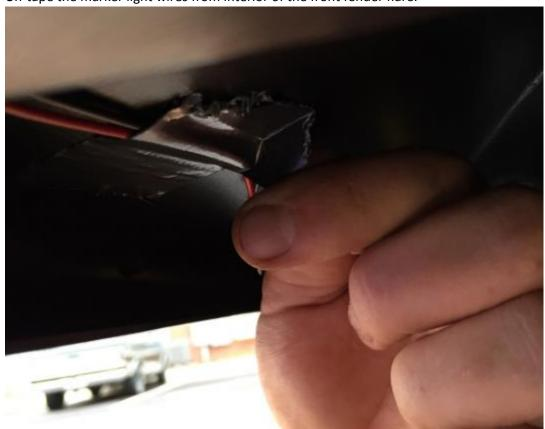
d. Pair each factory lead wire with the marker light wiring and twist the exposed fibers together.
