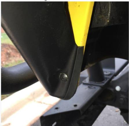
b. Now install screws with washers in the 3 positions closest to the door. Start at the bottom position, and work your way toward the center of the fender flare.
