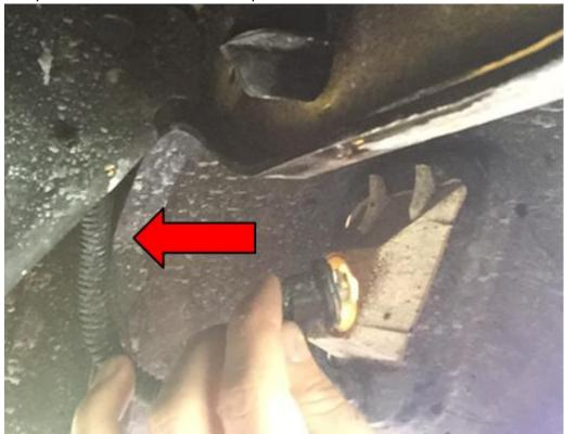
c. Remove the bolt at the front most position using an 8mm wrench or socket drive.
