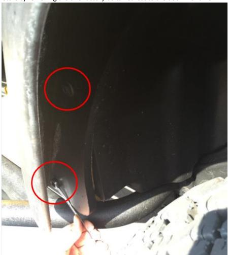
b. Remove the rear-most bolt using an 8mm socket drive.
