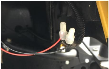
g. Using tape or a fastener of your choice, tuck the wires into a hidden space so that they are not handing from down in a visible area of the wheel well and secure their position. There is nothing supplied in the kit to aid you in hiding the wires, so the treatment is up to you. (Weatherproof tape is an inexpensive solution).
