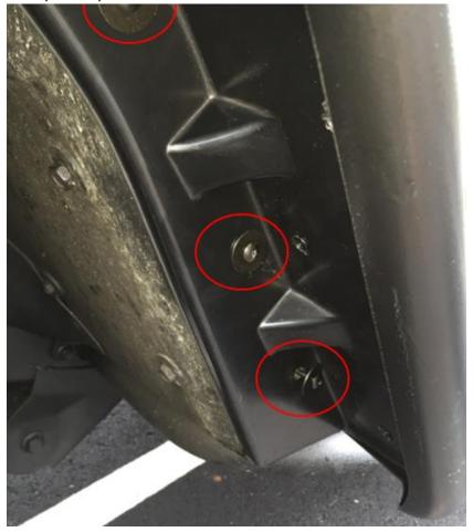
c. Now install screws with washers and flange nuts in all remaining positions on the front fender flare.
