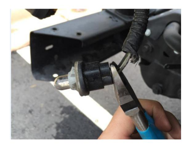
b. Using a pair of wire strippers, strip the end of each lead.
