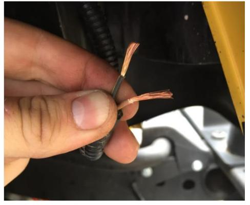
c. Un-tape the marker light wires from interior of the front fender flare.
