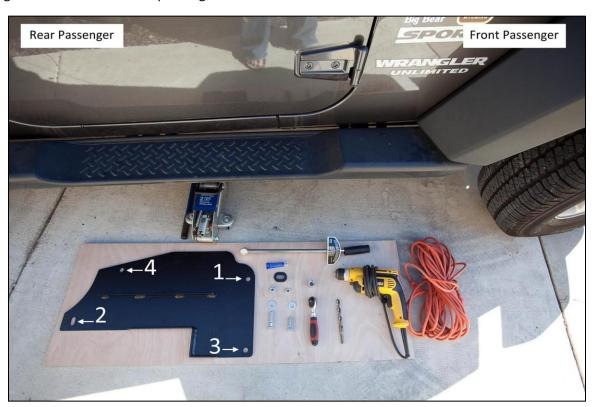
2. Remove factory bolt and washer set #1 and #2 using 18 mm socket and 3/8 inch socket wrench.
