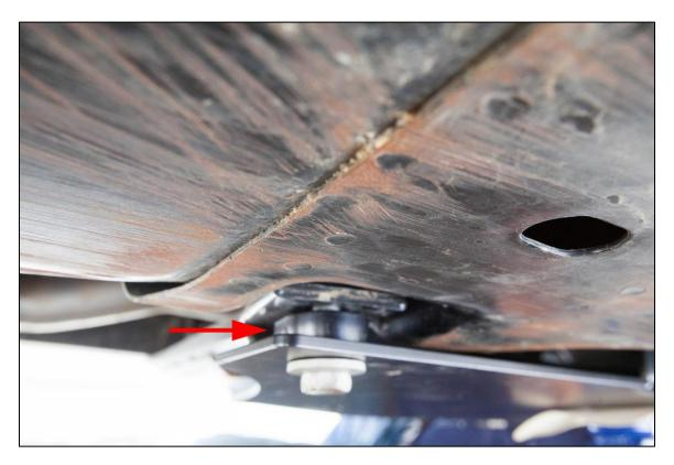
7. Using M.O.R.E skid plate holes #3 (cross member location) and #4 (factory skid plate location) as guides, drill two 9/16 inch holes.
