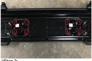
//Step 2: Remove the fog lights from the original bumper by removing (8) phillips head screws.
