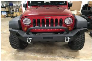
**//Step 7:** Install the 3/4" D-Rings into the front of the bumper, installation is now complete.
