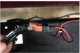
//Step 6: Plug the extension harness into the vehicles fog light harness. Once the harness is installed, plug the extension into the fog lights in the bumper.
