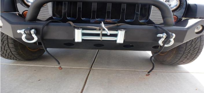
9. Run harness through frame work and reattach fog light plug to back of fog lights.
