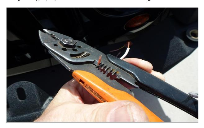
6. Connect and crimp both 20" to 24" #18 black wiring to plug and harness. Repeat step with 20" to 24" #18 white wiring.
