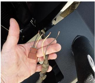
4. Using wire crimpers, crimp all 8 - #25 Butt Splice Crimp/Heat Shirk connectors (Waterproof) to end of fog light plug and harness.
