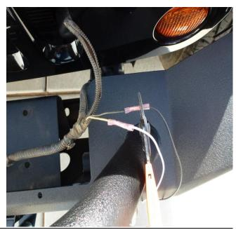
7. Using heat gun (Barbeque lighter will work) shrink all 8 - #25 Butt Splice Crimp/Heat Shrink connectors (Waterproof)
