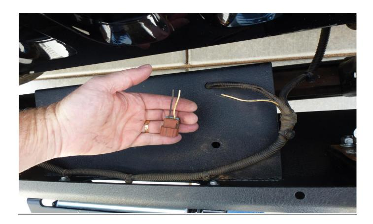
3. Using wire strippers strip both black and white wires on the plug and wire harness ends.
