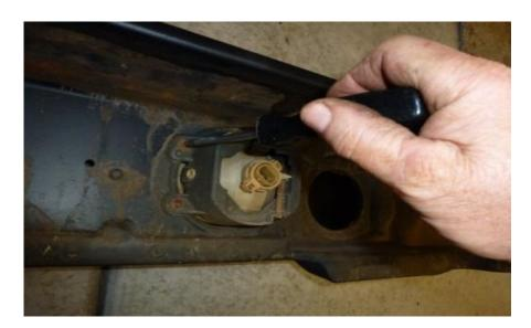
3. Place both fog lights on your new Barricade Trail Force HD Full Width Bumper. Use the provided screws and nuts for mounting. Use the Philips screwdriver and 7mm wrench to fasten screws and nuts (8 screws, 8 nuts).
