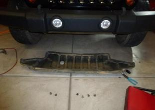
d) Remove both fog lights from back of OEM bumper using Philips screwdriver (8 screws in all).
