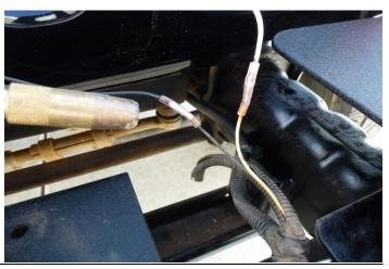
8. Cover with electrical tape and 3/8" flex tubing. The flex tubing will give it the OEM look you are looking for.
