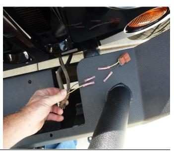
5. Using wire strippers, strip both ends of #18 20" – 24" black and white wiring.
