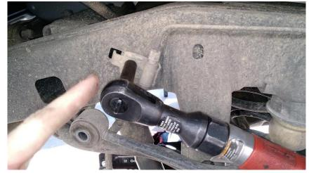
7. Using needle nose plyers, undo the little plastic clips (picture 1) securing the wheel speed sensor wire so the hanging axle doesn't stretch it. Using a 10mm socket remove both nuts holding the emergency brake bracket to the bottom of the tub (picture 2), so the axle can hang freely.
