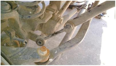
13. Use cable ties or Zip ties to tie the lower brake mounting bracket to the lower end of the shock. This bracket used to be connected in front of the shock absorber (where I am pointing) and has now been routed behind it. Note: you may remove this bracket from the brake line, but proceed with extreme caution. One wrong move and you'll be buying a new brake line.
