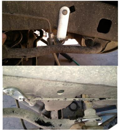
12. Raise the axle up and Compress the shocks by hand in order to line them up to be installed with the shock extension brackets. Compress the shocks as needed to fit the extension brackets in and loosely thread the 10mm x 80mm bolts in before tightening.
