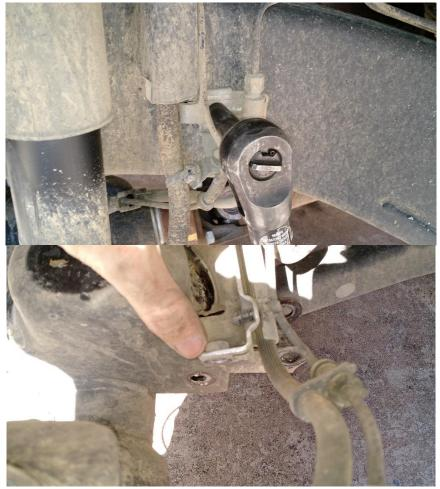
6. If the axle is not drooping enough to remove the springs, use the teeter totter method, have someone stand on one side of the axle and jack up the other side of the axle until you can pull the spring and isolator from its position.
