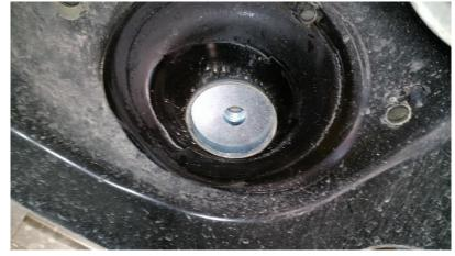
10. Use the open end of a 19mm wrench to hold the rear spacer retainers still, install the rear coil spacers with the supplied ½" x 2 ¾" bolt and lock washer. Install the spring isolators on top of the springs and wiggle the springs back into place. There are no spring stops on the rear axles, but make sure the springs are matching/rotated the same way.
