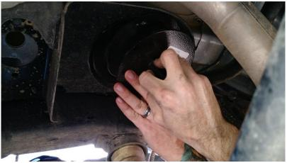
11. Install the Brake line bracket using a 10mm socket with the original hardware and 11mm socket/wrench on both sides of the new .250-20 x 1" bolts, washers, and nuts on bottom. I recommend installing the bottom on the back side of the bracket (inside of frame) due to clearance with the rear sway bar. See clearance of upper link bolt in picture 2.
