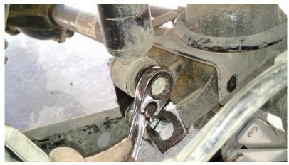
12. Looking at the sway bar end link at full droop, this is a great reason to buy "quick disconnect" sway bar end links from ExtremeTerrain. If longer end links are not used, at full droop, you run the risk of flipping the sway bar forward, bending suspension equipment or breaking the Rubicon's electronic disconnect motor. Always disconnect on the trail, and reconnect the end links when back on level pavement.
