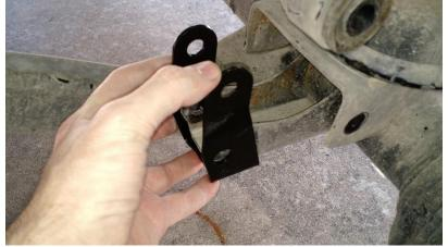
10. Use the large 12mm x 65mm bolts and small 5/16" x ¾" bolts to secure the bracket to the original mount on the axle. Tighten using an 18mm socket/wrench on either side for the large bolt and a 1/2" socket/wrench on either side of the small bolt.
