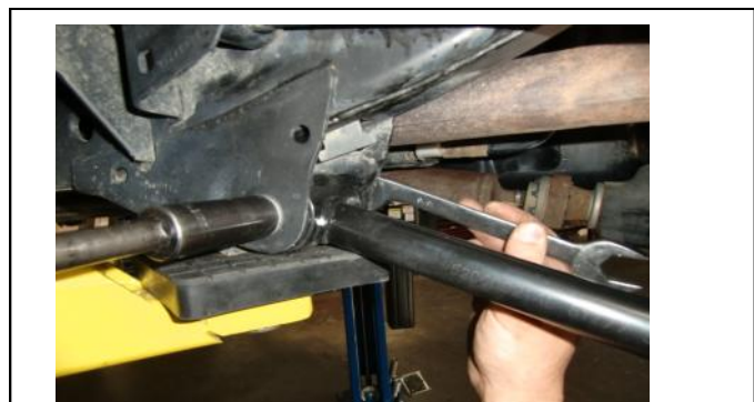
4. Unbolt the Drivers side rear lower link from the frame and remove.
