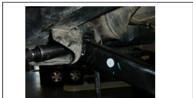
4. Unbolt the Drivers side front lower link from the frame and remove.
