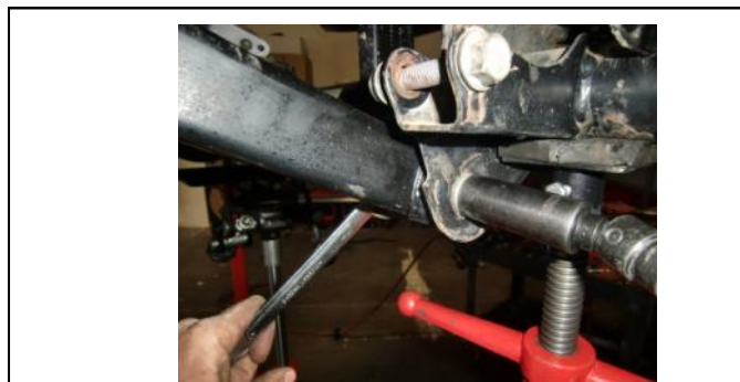
3. Support the front axle. Work on one side of the vehicle at a time. Unbolt the drivers side front lower link from the axle side.
