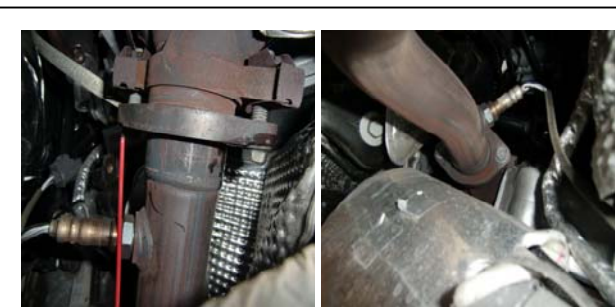
16. On passengers side, unbolt the header from the exhaust. Use some type of thread lubricant to help free rusted exhaust.
