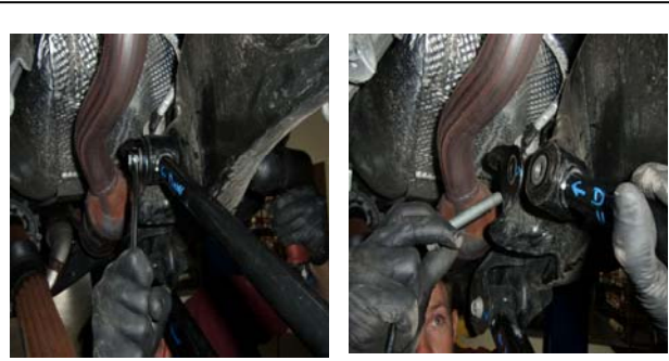
14. Unbolt drivers side front upper arm from the frame.
