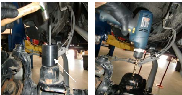
20. Center, mark and drill 7/16 hole.
