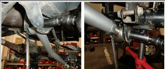
19. Install the new front lower arm on both sides of vehicle and tighten. The adjustable end should be mounted at the axle and the bend should point to the center of the vehicle also badges should be legible.
