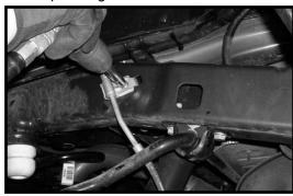
Working on the driver side, install the stock shock into the stock lower mounting location and secure using the stock hardware. Make sure to use thread locker or loctite and torque to 65 ft lbs. Repeat procedure on the passenger side.
