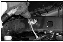
23. Locate the stock lower shock mounting hardware. Working on the driver side, install the stock shock into the stock lower mounting location and secure using the stock hardware. Make sure to use thread locker or loctite and torque to **65 ft lbs.** Repeat procedure on the passenger side.
