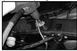
18. Working on the driver side, carefully remove the stock ABS line clip from the bottom side of the stock frame rail. Special note: Take special care not to damage the ABS line clip during removal. This will need to be reinstalled back into the same hole at a later step. Repeat procedure on the passenger side.
