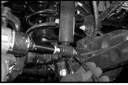
5. Carefully lower down on both hydraulic floor jacks until the front coil springs can be removed. Working on the driver side, remove the stock coil spring. Set aside for later reinstallation. Repeat procedure on the passenger side. Special note: Make sure to keep the driver and passenger side coil springs separate from each other. We need to make sure that the driver side coil spring gets installed back into the vehicle on the driver side and the same with the passenger side.
