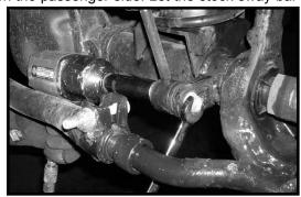
4. Working on the driver side, remove the stock mounting hardware that connects the stock shock into the stock lower mount. Save the stock hardware for later re-installation. Repeat procedure on the passenger side. Special note: There is no need to remove the shock completely from the vehicle. Keep the stock shock mounted to
