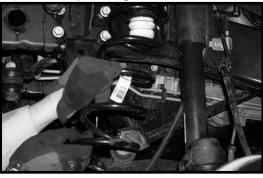
6. Locate the new front coil spring spacers. Working on the driver side, install the new coil spring spacer over the stock bump stop cup. Repeat procedure on the passenger side.
