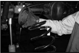
20. Locate the new rear coil spring spacers. Also, locate the stock driver and passenger side coil springs. Working on the driver side coil spring, place the new rear coil spring spacer on top of the stock coil spring and install the stock coil spring and new rear coil spring spacer back into the stock location. Repeat procedure on the passenger side. Carefully raise up on both hydraulic floor jacks until the stock coil springs and spacer seat properly into the upper and lower locations.
