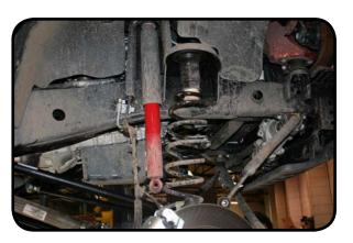
18. Remove sway bar links using 18mm socket and wrench at the axle and 18mm socket and 20mm wrench at the sway bar. Lower the jack enough to remove the springs.
