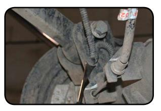
Remove the bracket that holds the park brake cables to the body using a 10mm deep well socket.
