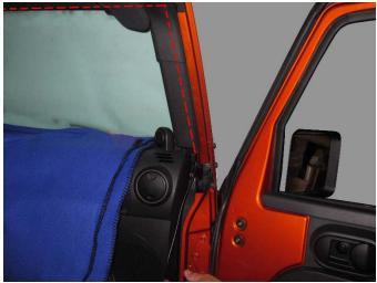
**Step 6:** Plug the rearview intermediate wiring into the rearview mirror.
