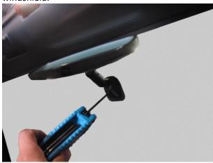
**Step 2:** Place the new mirror over the metal windshield mount and slide it down. Tighten the T20 Torx screw, until snug.
